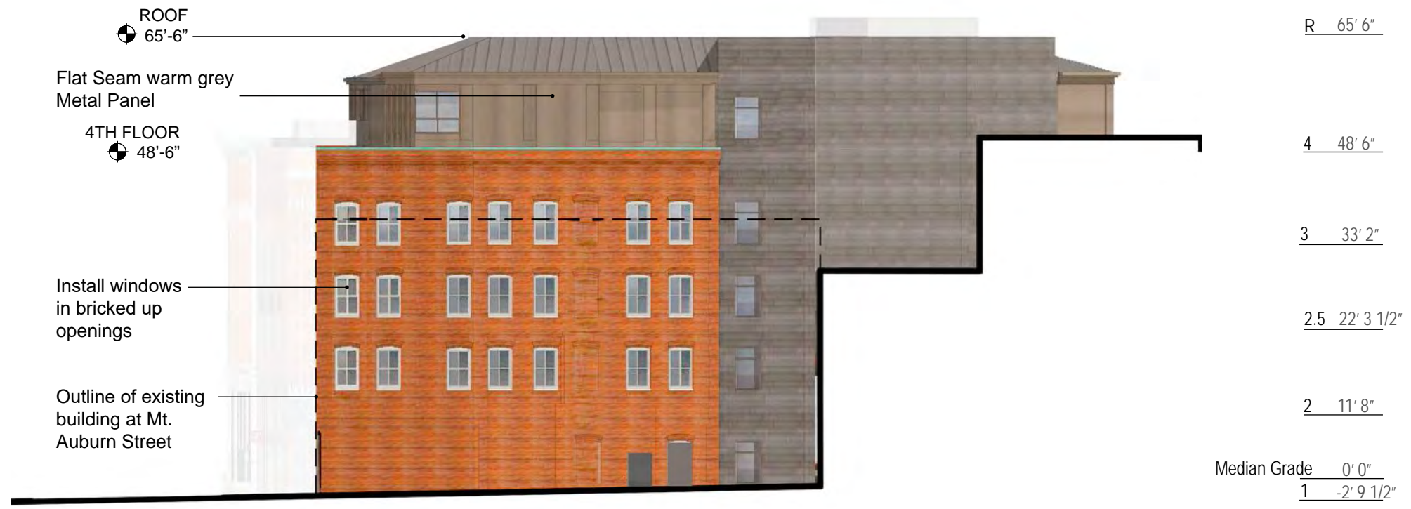
WEST ELEVATION (INTERIOR TO THE BLOCK)
