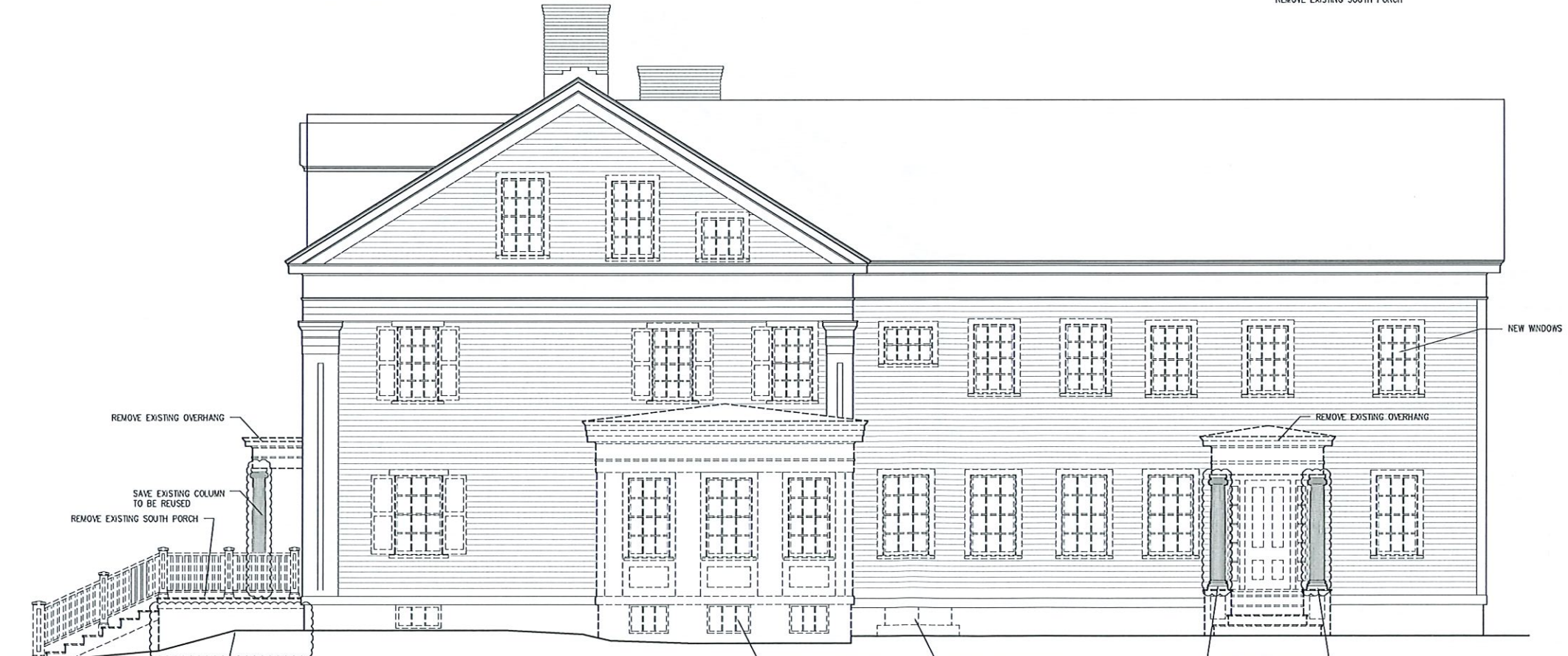
2 DEMOLITION EAST ELEVATION SCALE: 1/4" = 1'-0"
