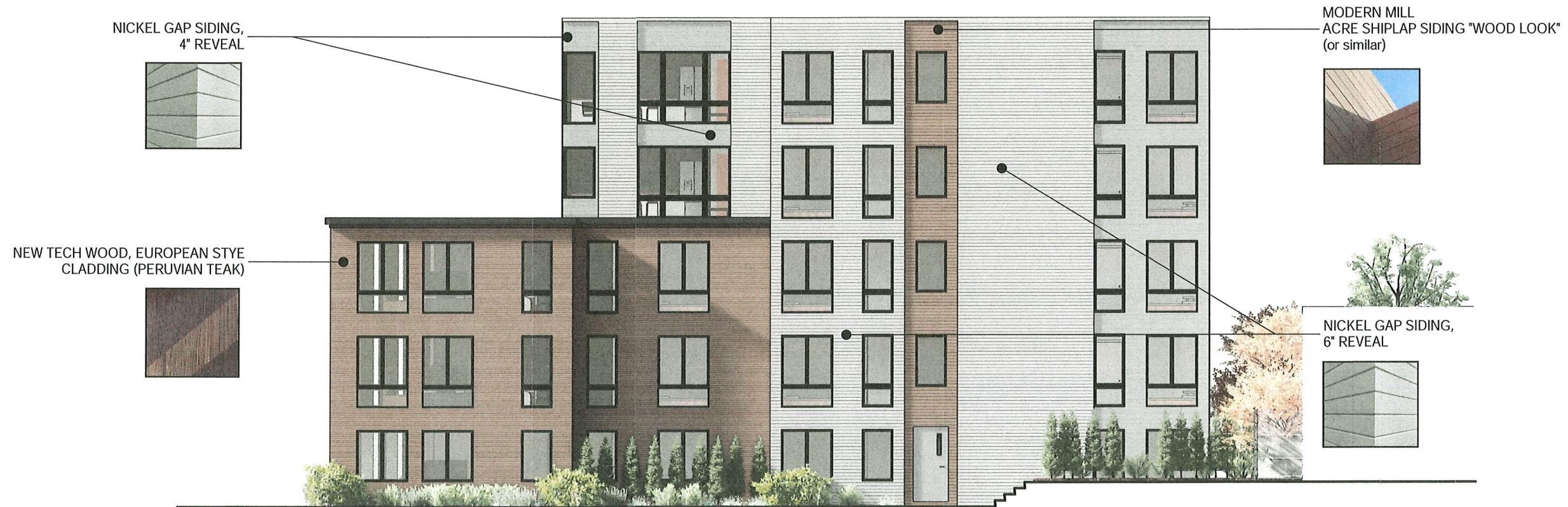
① Side Yard Elevation 3/16" = 1'-0"
