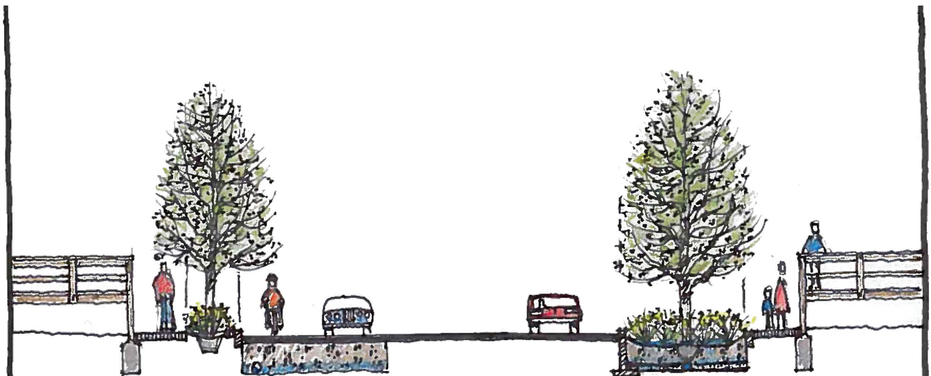
A street section from the CCPR Plan demonstrates the integration of stormwater management and resiliency features into the streetscape (see Mobility section on page 130-131 for detailed street sections).
