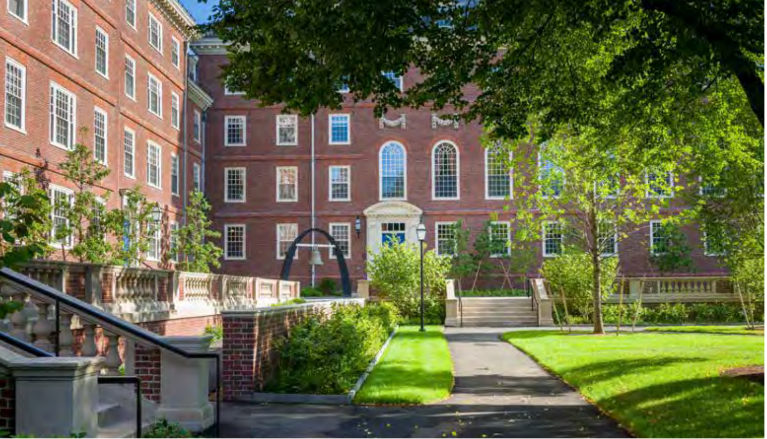
The landscape of the central courtyard was restored to something more closely resembling its original appearance. The existing configuration of pathways was largely retained, however they were modified slightly to reflect new building circulation patterns and re-graded for accessibility and to restore proper site drainage.
