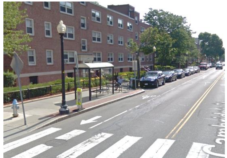
Example of a curb extension with a bus shelter on Cambridge Street.
