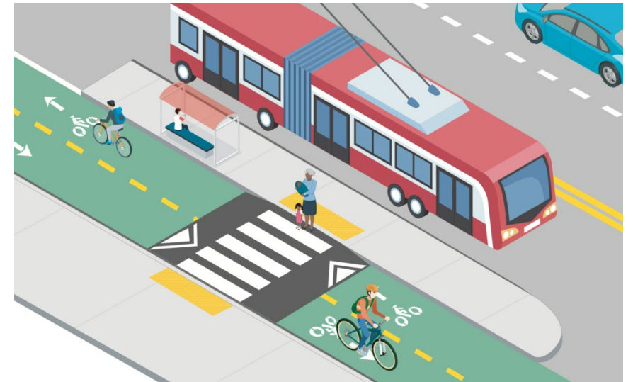
Above Cartoon showing a bus boarding island with a raised crosswalk with a two-way separated bike lane. Shows a trolleybus that would not be found on this section of Huron Avenue. Illustration by Eric Tuvel.
