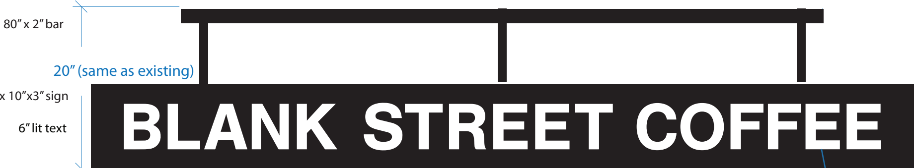
2 Front View- Pan Sign w/ Raised Lit Letters - 7.08 Square feet 1" scale Note: same lighting method as existing sign
