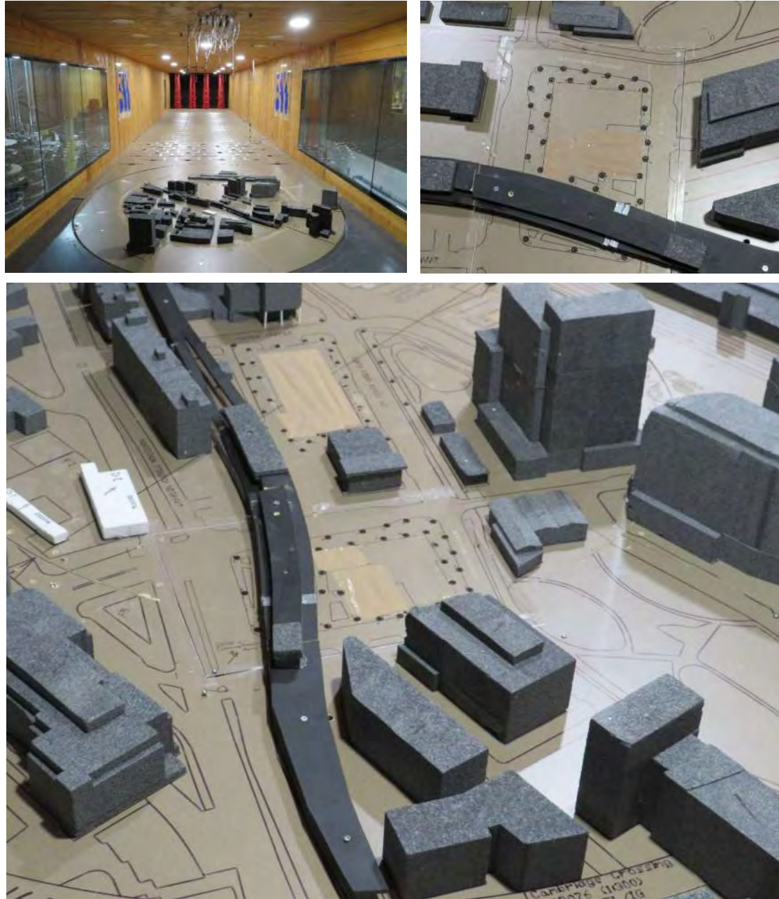
Image 2A: Wind Tunnel Study Model - Existing Configuration
