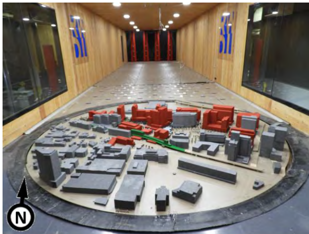
Image 2: Wind tunnel study model - proposed configuration
