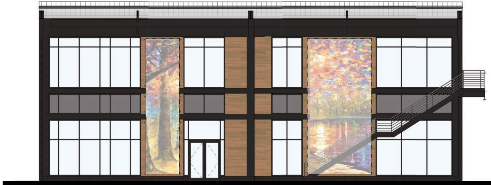
South Plaza Elevation - Tensile hanging system with large format artwork
