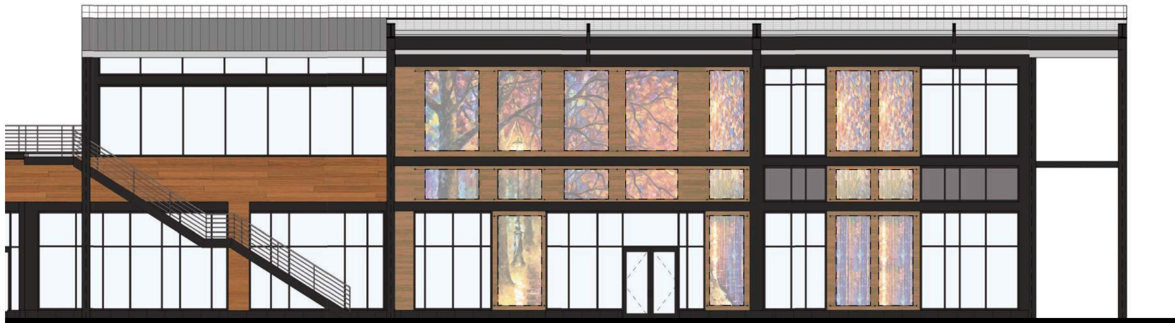
North Plaza Elevation - Tensile hanging system for flexible artwork size & location
