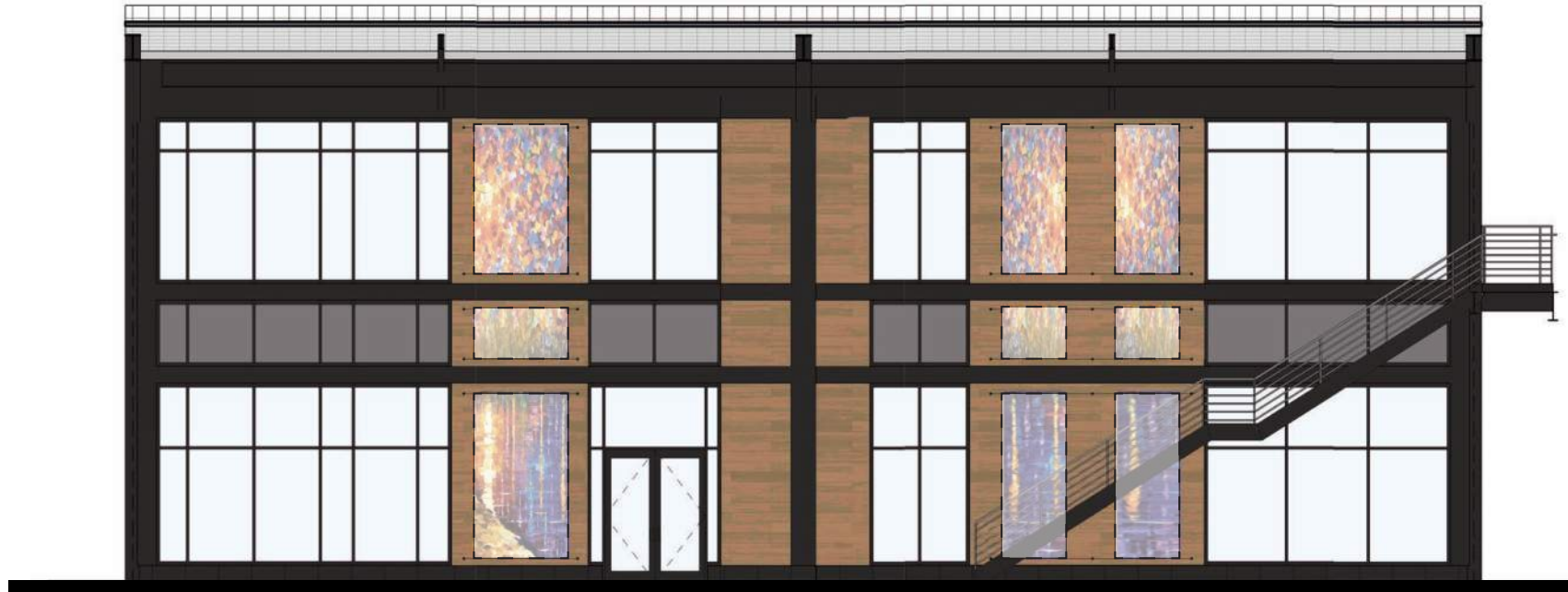
South Plaza Elevation - Tensile hanging system for flexible artwork size & location
