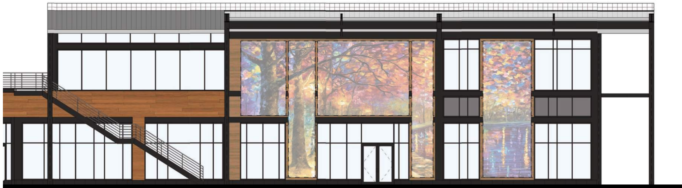
North Plaza Elevation - Tensile hanging system with large format artwork
