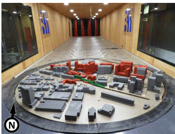
Image 2: Wind tunnel study model - proposed configuration
