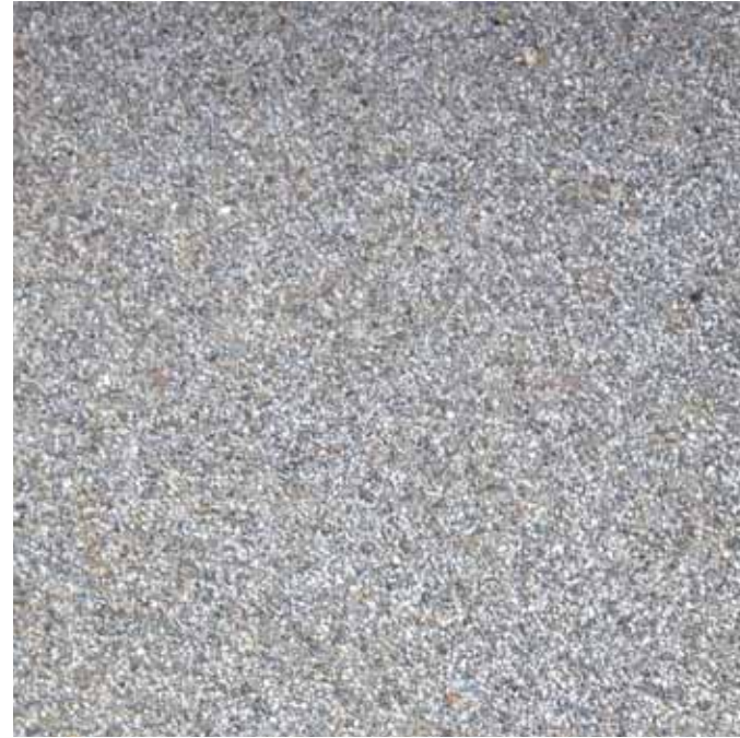
Exposed Aggregate Concrete Pavement
