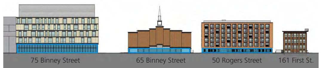
Main volume of buildings above a ground floor base
