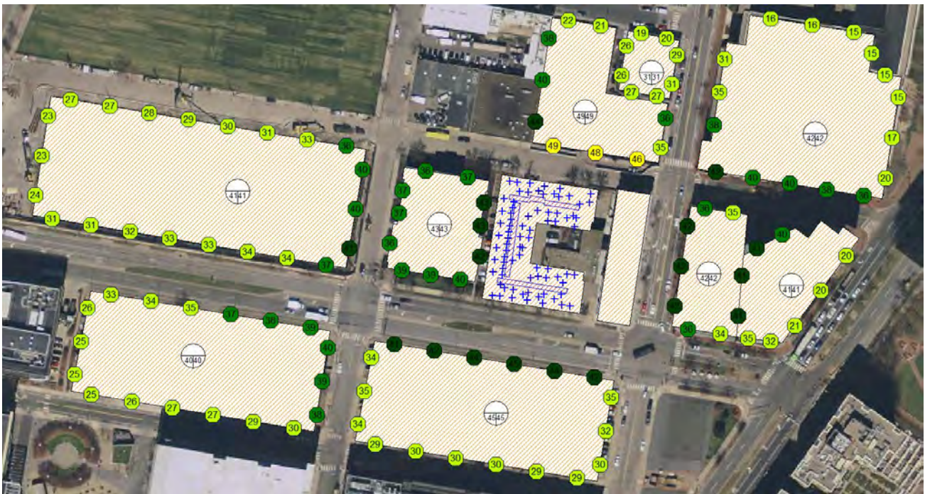
FIGURE 2. A-weighted sound levels produced by building mechanical systems
