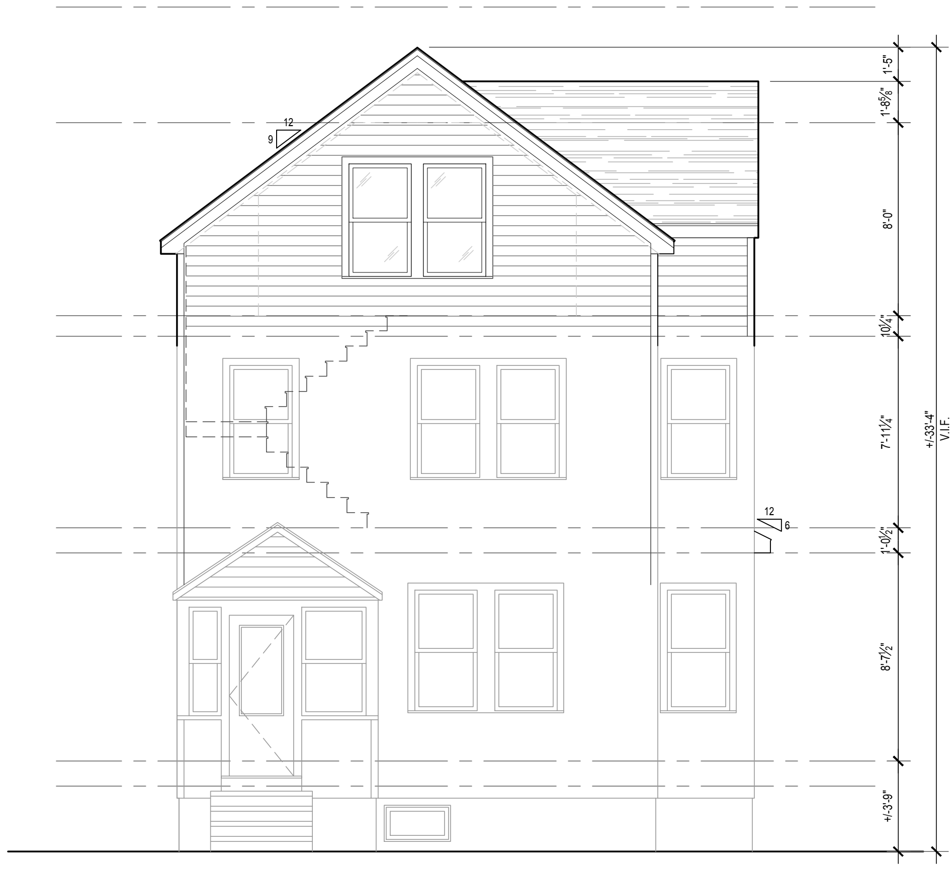
1 NEW EXTERIOR ELEVATION: FRONT 1/4" = 1'-0" SOUTH FACING
