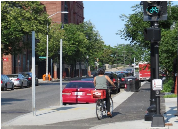
Signalized bike crossings
