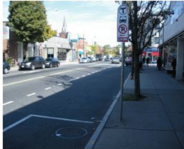
Curbside pull out stop in parking lane
