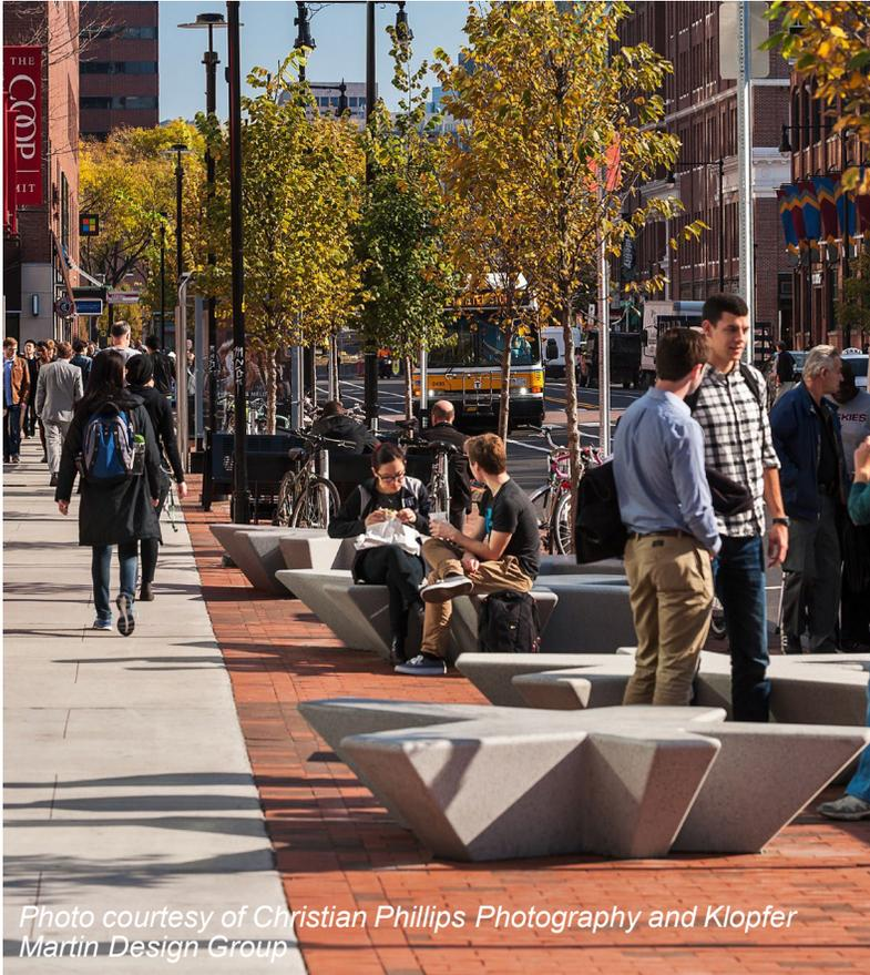
Concrete and wire-cut brick without beveled edges, placed on a smooth asphalt base, will be utilized as the sidewalk materials of choice throughout the City. Concrete is the material most frequently used in the city (~70%) and provides a relatively inexpensive, durable, and easy-to-maintain accessible sidewalk.
