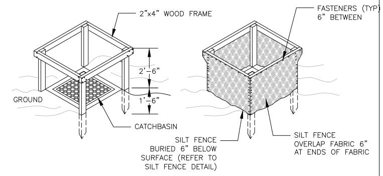
THIS METHOD OF INLET PROTECTION IS APPLICABLE WHERE THE INLET DRAINS A RELATIVELY FLAT AREA (SLOPE NO GREATER THAN 5%). WHERE THE INLET ACCEPTS SHEET OR OVERLAND FLOW (NOT GREATER THAN 1 CFS) ARE TYPICAL. THE METHOD SHALL NOT APPLY TO INLETS RECEIVING CONCENTRATED FLOWS
