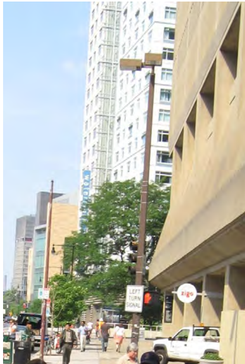
Shoebox luminaires used in Kendall Square for both roadway and pedestrian scale lighting
