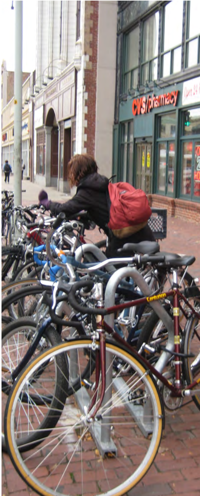
Figure 7.4: The “Swerve” rack on a rail system enables racks to be located where it is not feasible to drill into pavement.
