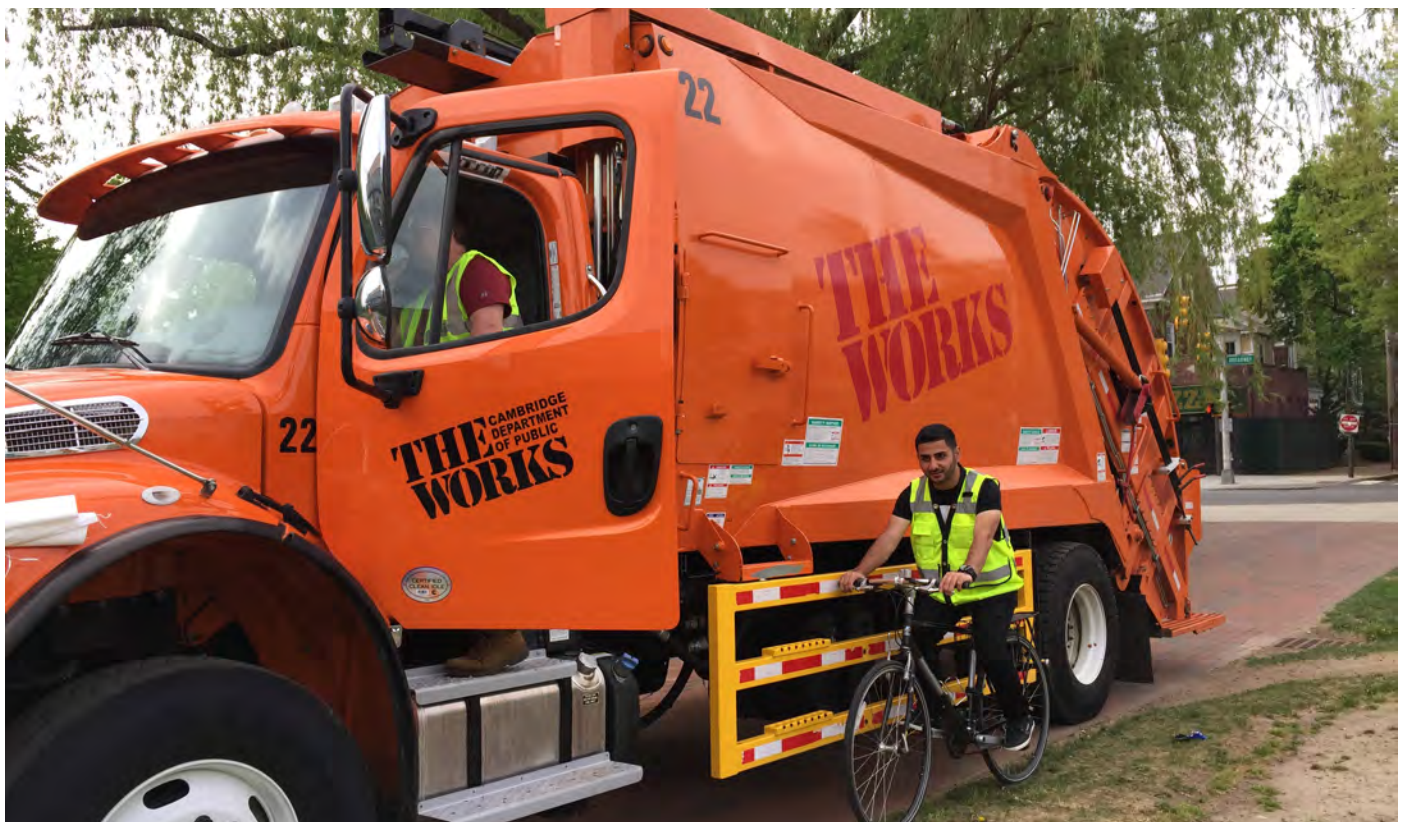
Cambridge Department of Public Works employees demonstrating truck side guards on City trucks.
