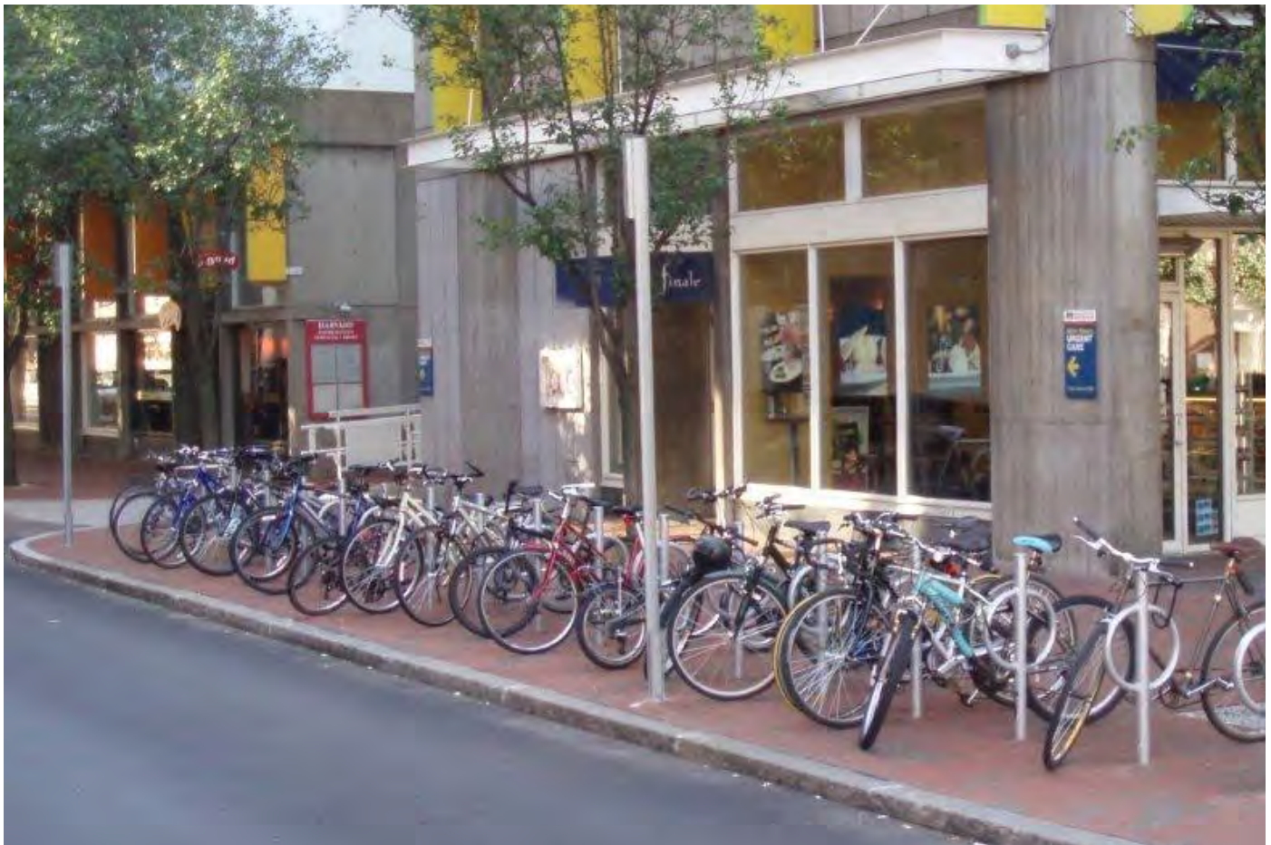
Figure 7.1: Curb extensions are sometimes built in order to provide space for added bicycle parking, and the “post and ring” model has a compact footprint.
