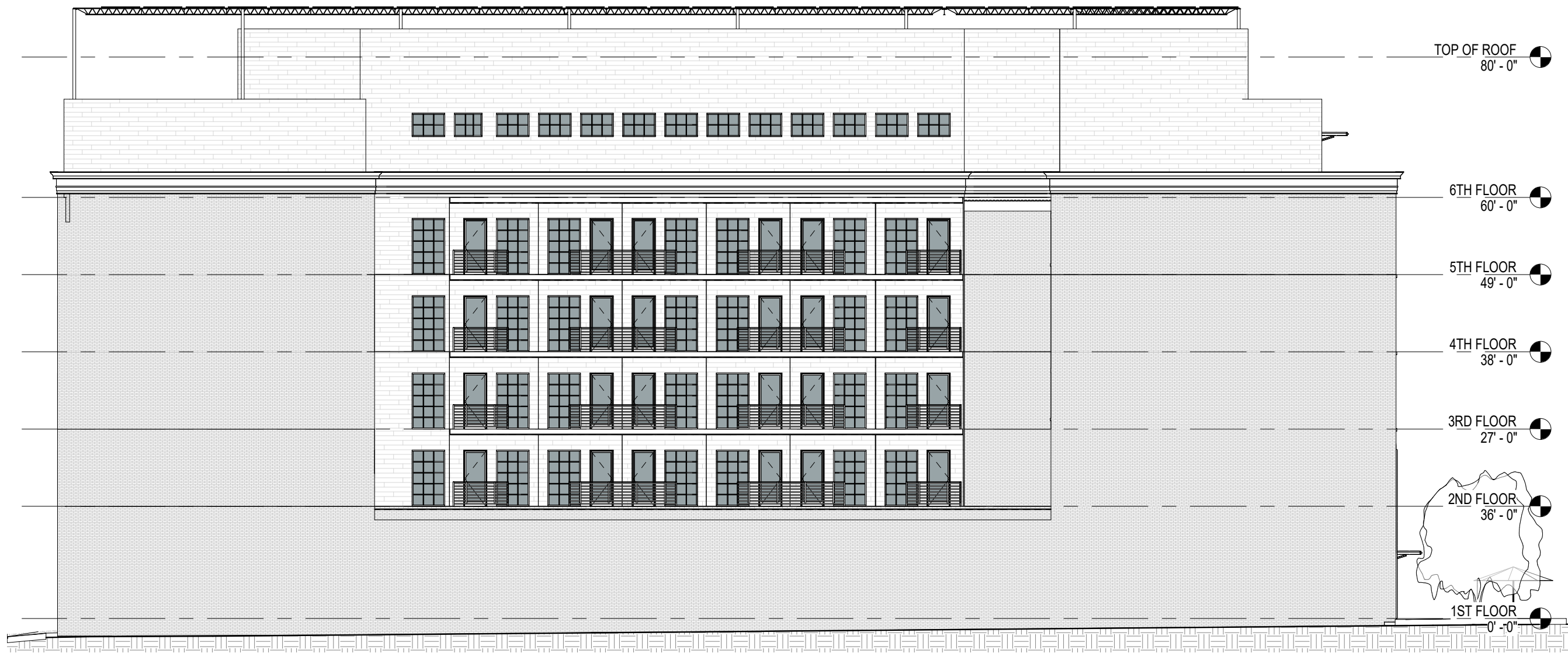
MASS AVE LEFT SIDE ELEVATION 1/16" = 1'-0"
