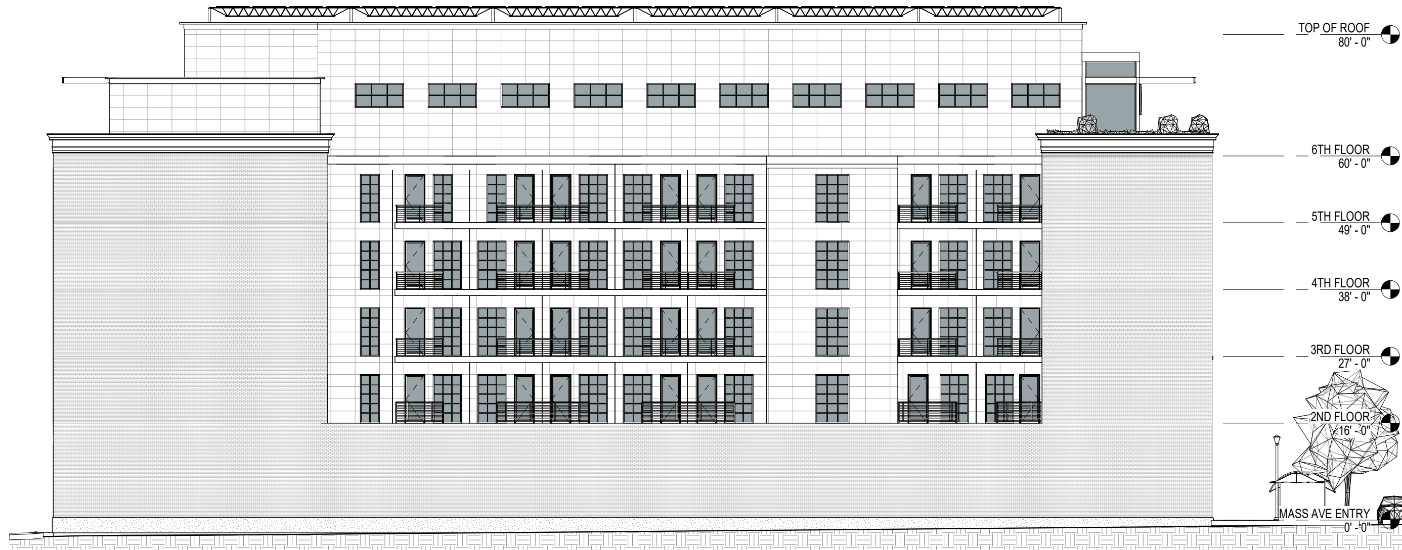
MASS AVE LEFT SIDE ELEVATION 1/16" = 1'-0"
