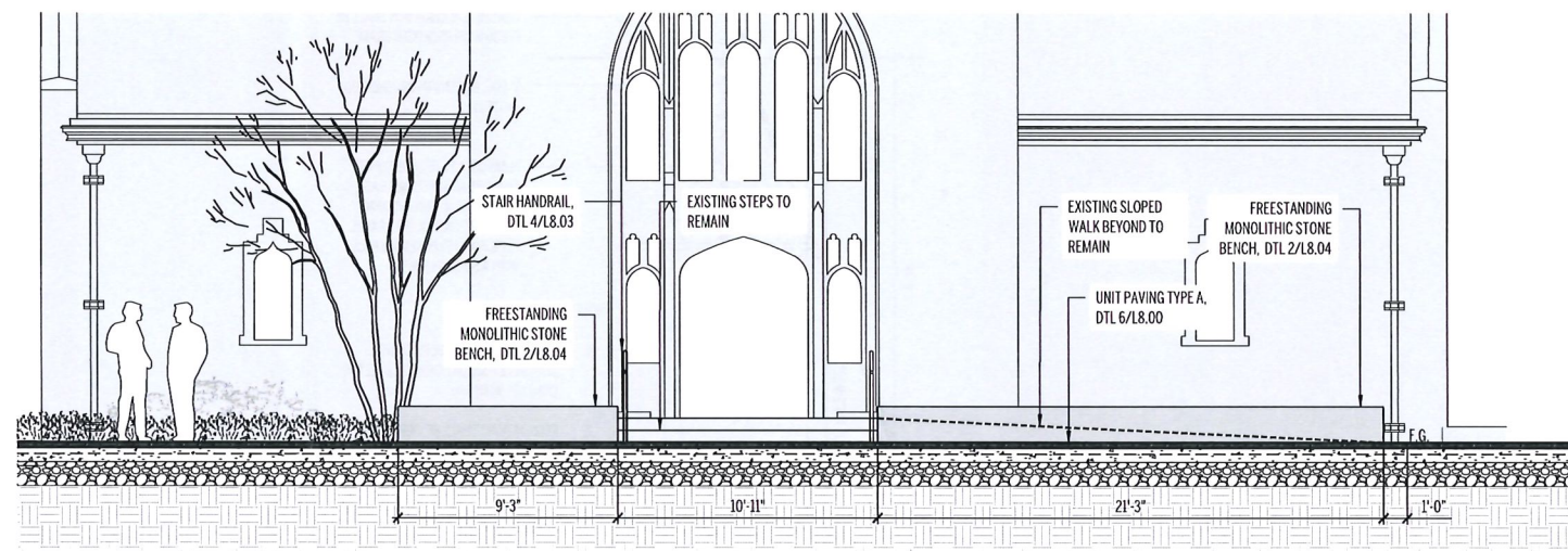
2 SECTION B: GRANITE TERRACE AT WRIGHT HALL 1/4"=1'-0"
