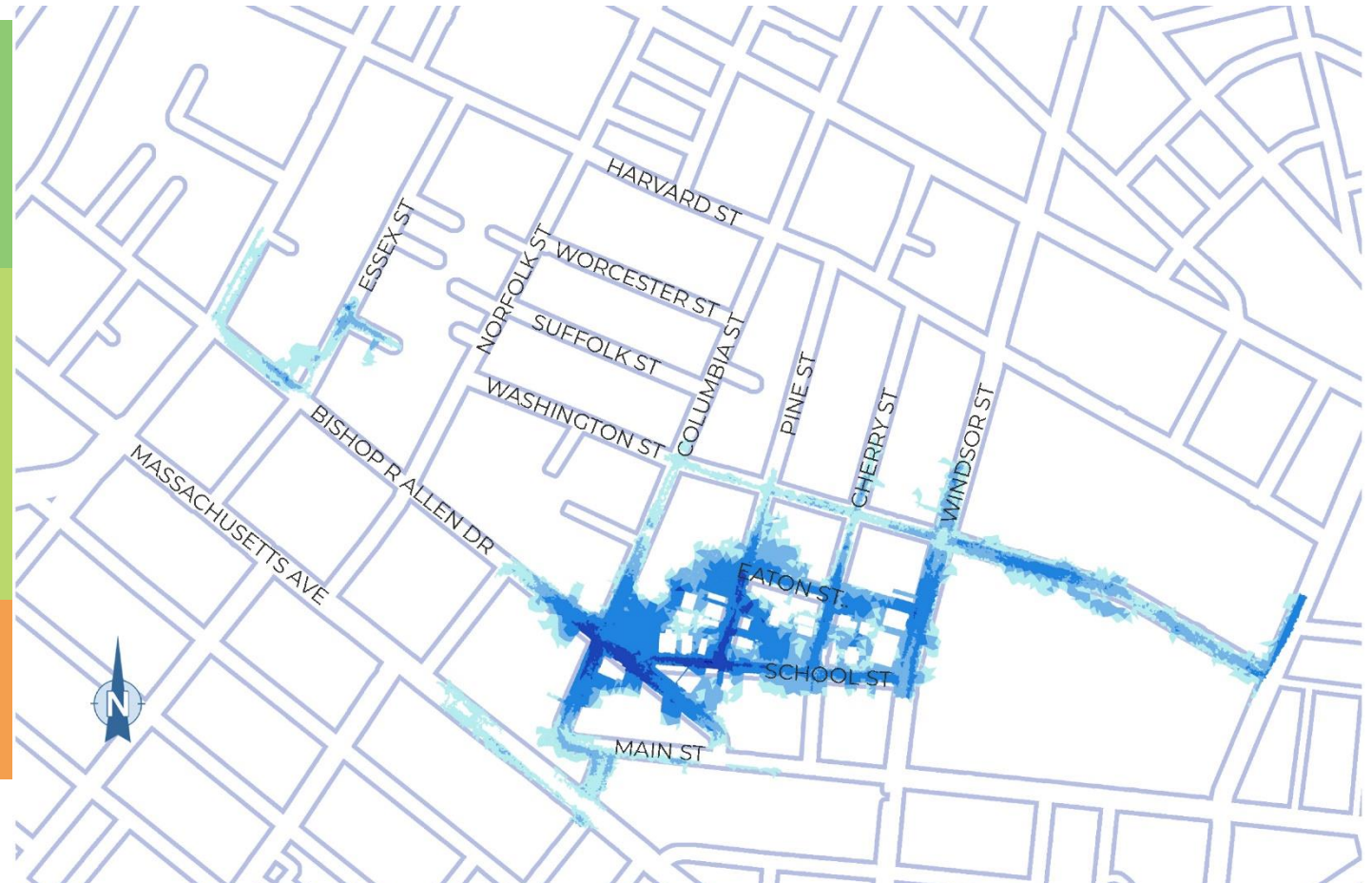
Anticipated flooding for a 2030, 10 year / 24 hour storm
