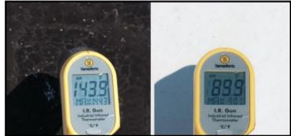
Figure 1: Dark vs. Cool Roof Surface Temperatures
