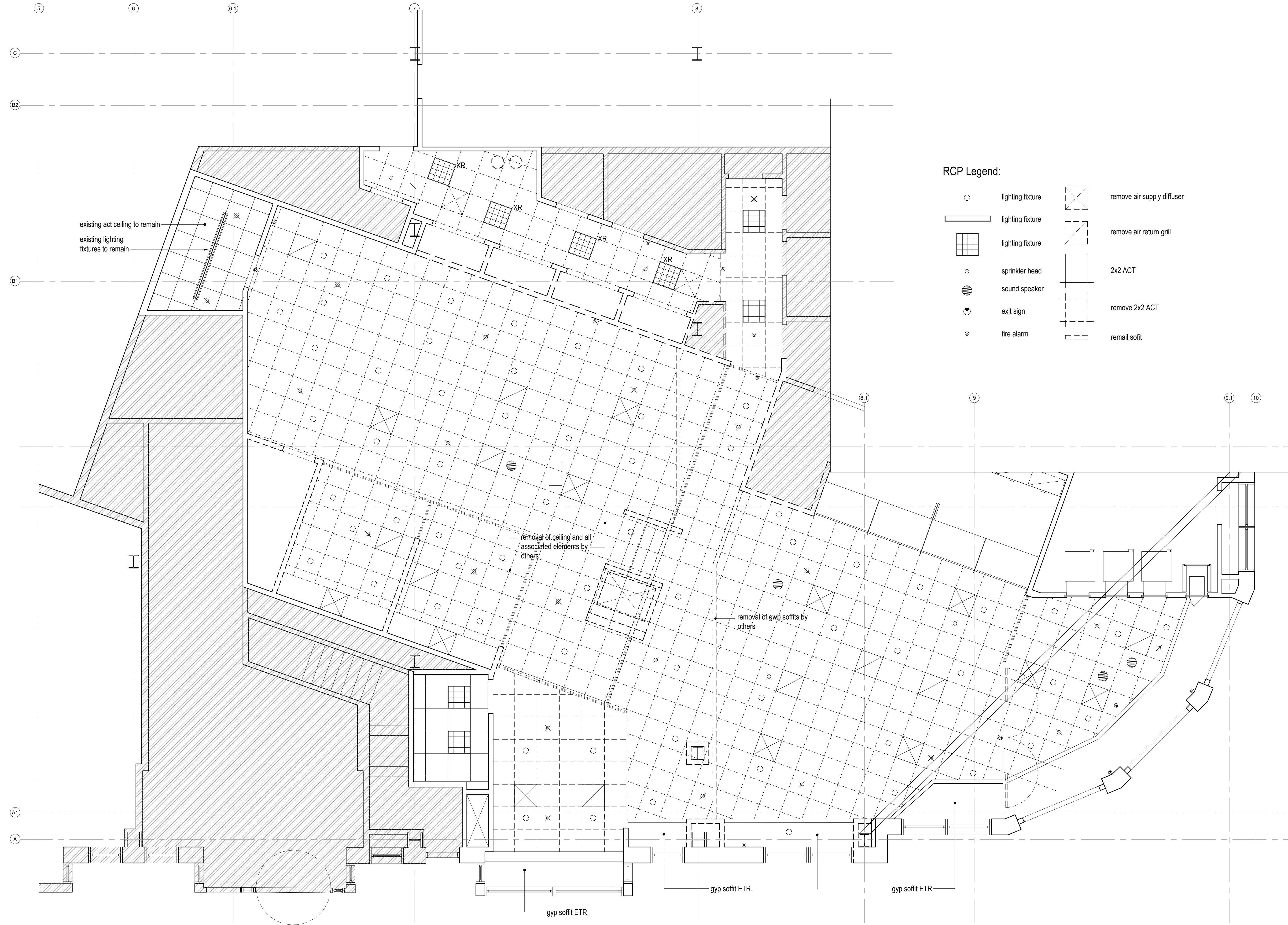
1 Demolition Reflected Ceiling Plan
