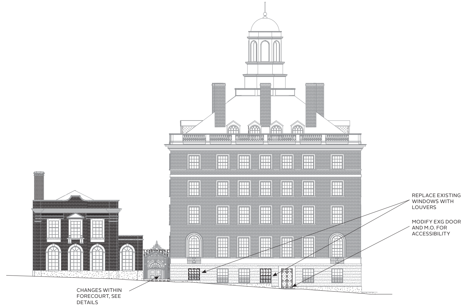
EXISTING/DEMO WEST ELEVATION
