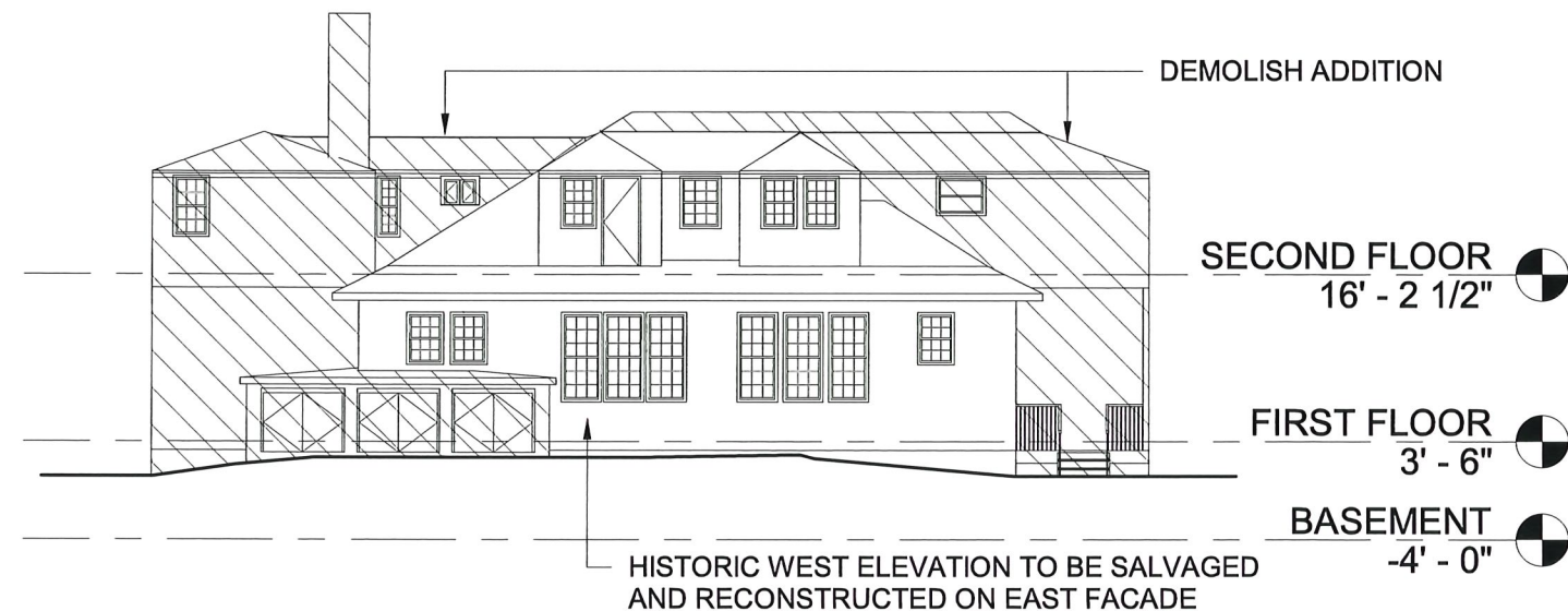
4 DEMOLITION - WEST ELEVATION M021 Scale: 1/16" = 1'-0"
