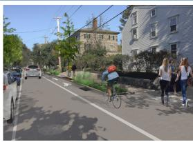
4-foot rain garden/bio-swale is provided on the east side, along with a 5-foot sidewalk. On the west side, a 3-foot zone for stormwater tree filters is provided, along with a 4-foot sidewalk.
