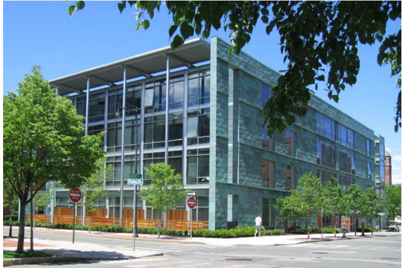
Emphasize the civic importance of primary public spaces by differentiating between front facade and side elevation by means such as contrasting materials, colors, scales, the amount and type of detail and articulation, and compositional formality vs. informality.
