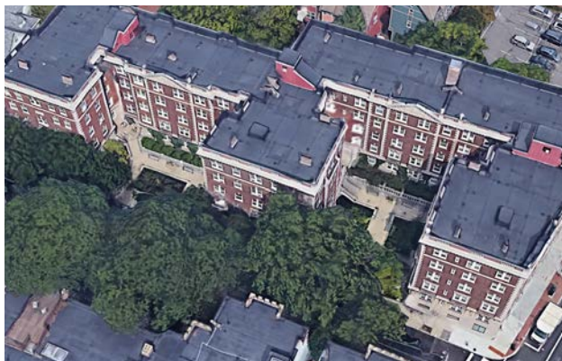
Large developments should include semi-public forecourts to break up long building facades.
