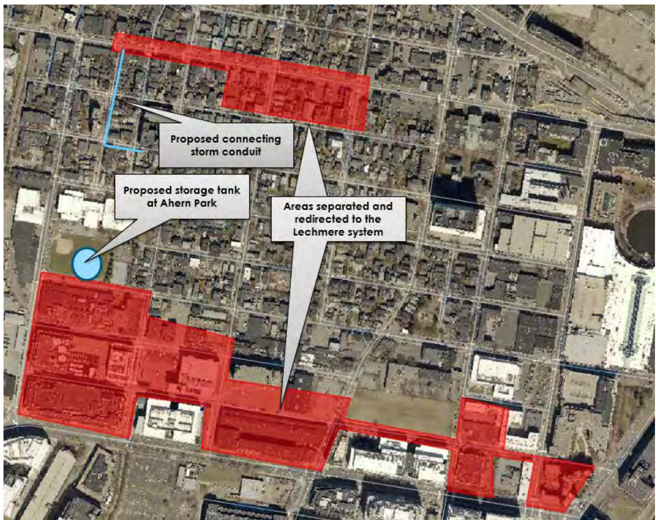
Figure 4. Alternative 3 proposed separation and redirection area and location of proposed storage tank
