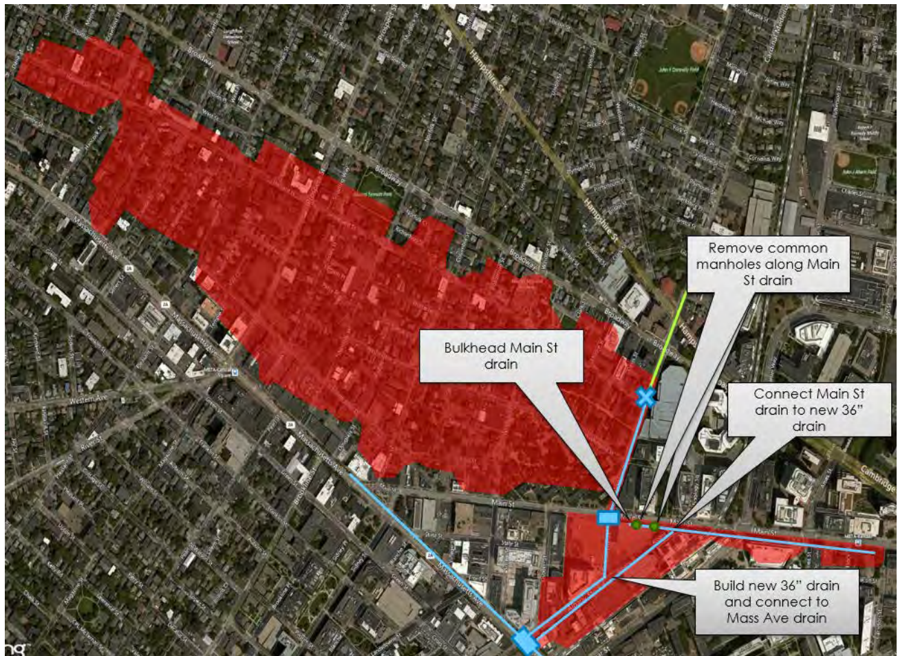
Figure 7. Actions needed for Alternative 6 (beyond Alternative 1) and separated area tributary to the Mass Ave drain
