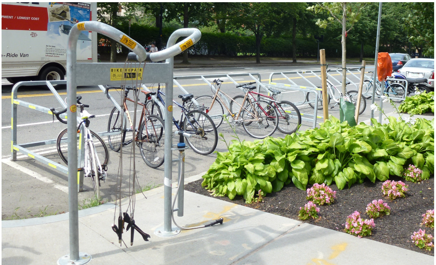
Figure 7.5: Example of a public repair stand and on-street bike corral located in Kendall Square.
