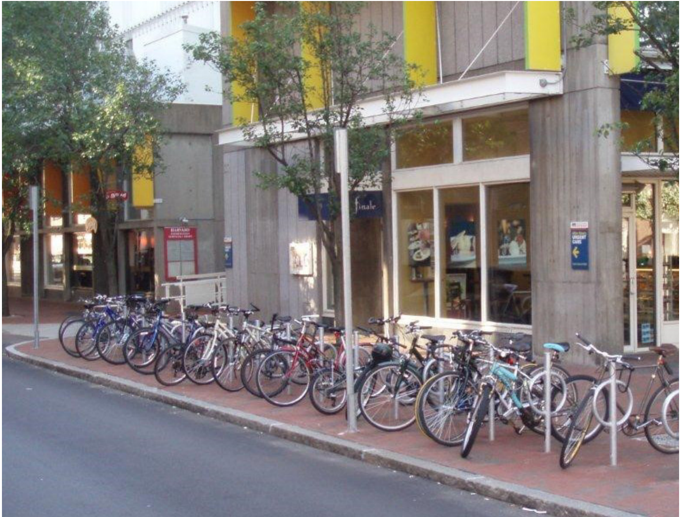
Figure 7.3: Curb extensions are sometimes built in order to provide space for added bicycle parking, and the “post and ring” model has a compact footprint.
