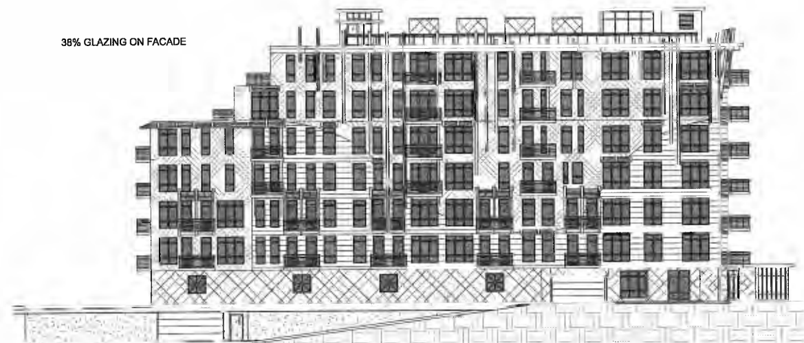
① Elevation 1 Glazing % 1/16" = 1'-0"
