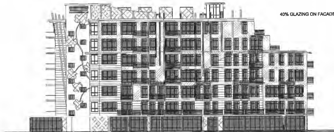
③ Elevation 3 Glazing % 1/16" = 1'-0"
