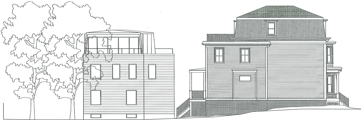
2 LEFT SIDE SITE ELEVATION 3/32"=1'-0"
