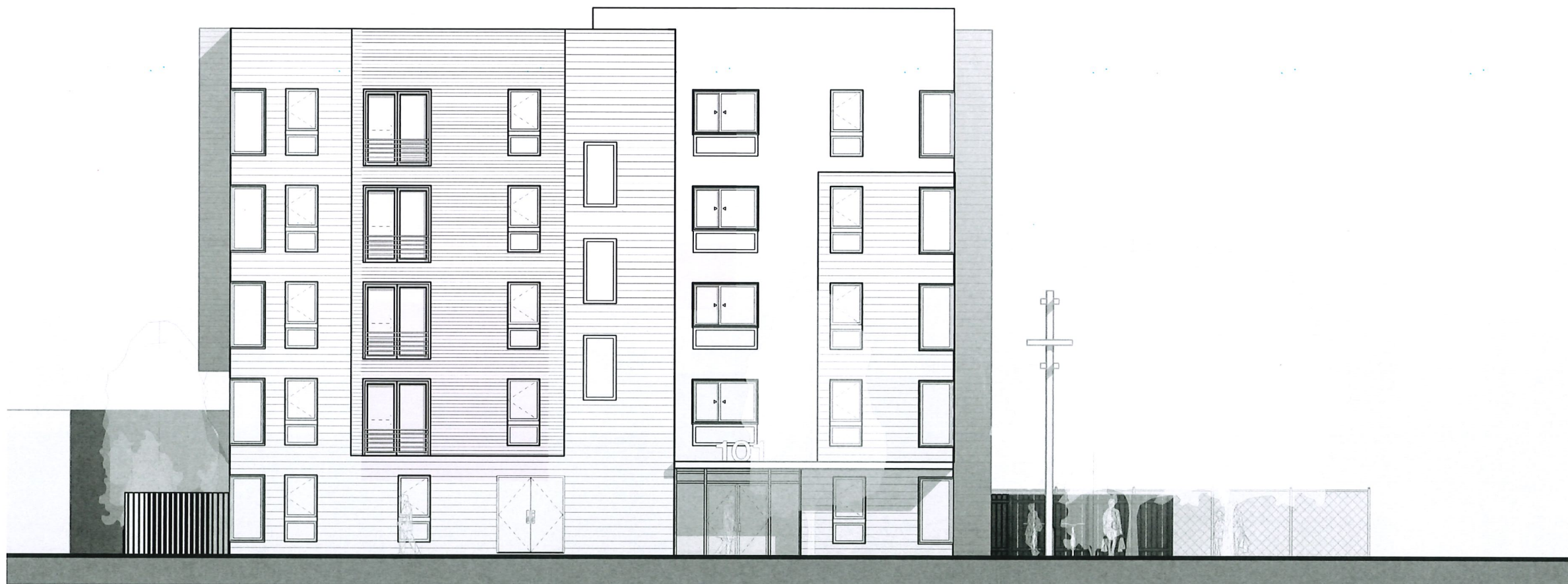
② BENT STREET ELEVATION 3/16" = 1'-0"
