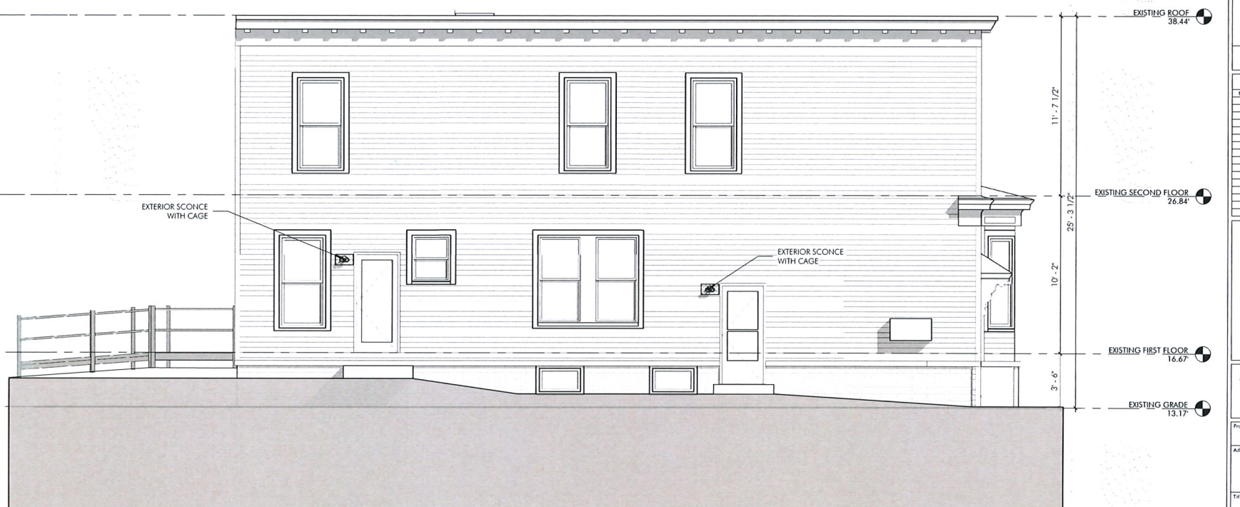
④ EXISTING NORTH ELEVATION 1/4" = 1'-0"
