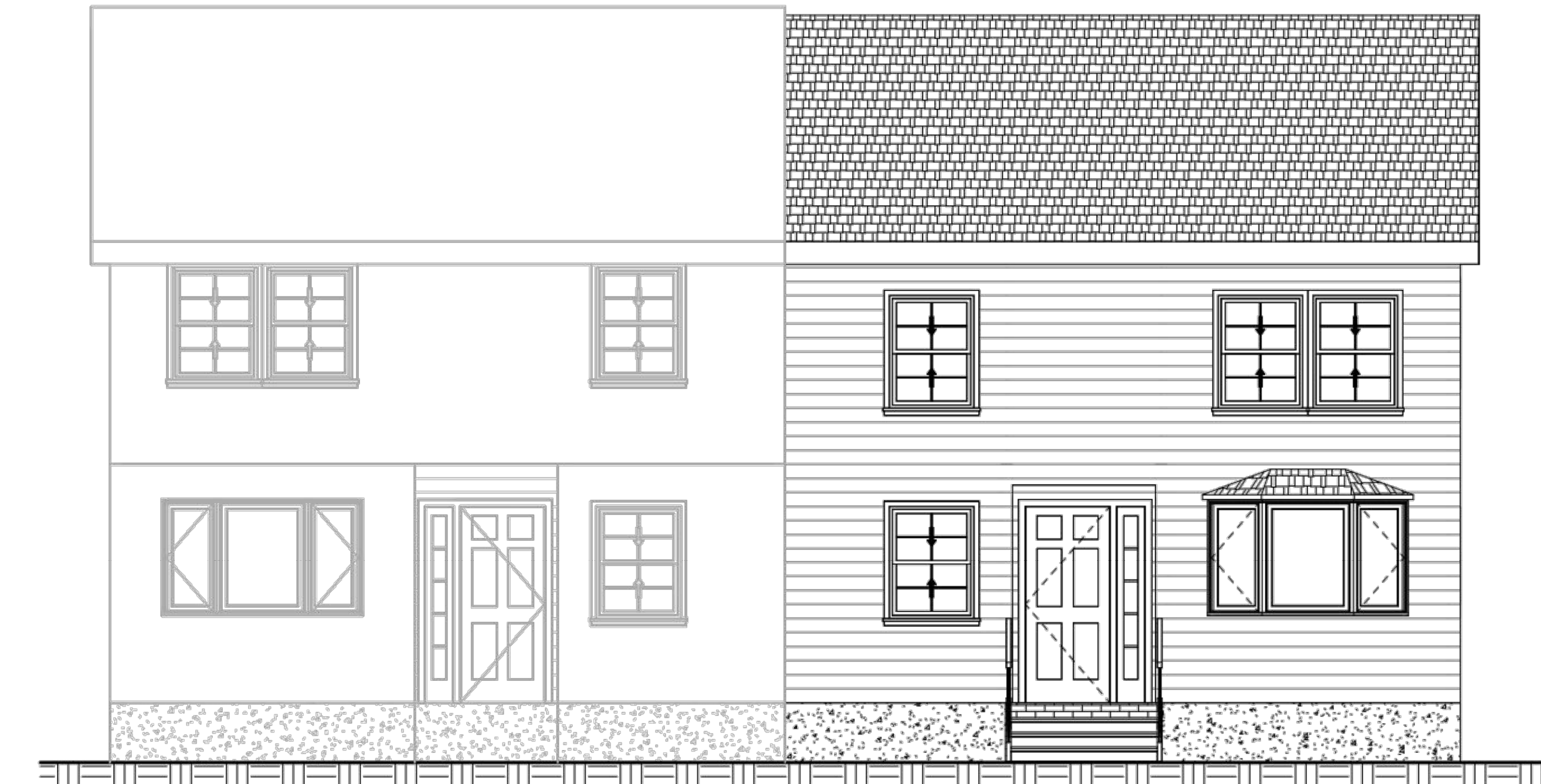
① FRONT ELEVATION - NORTH ELEVATION 1/4" = 1'-0"
