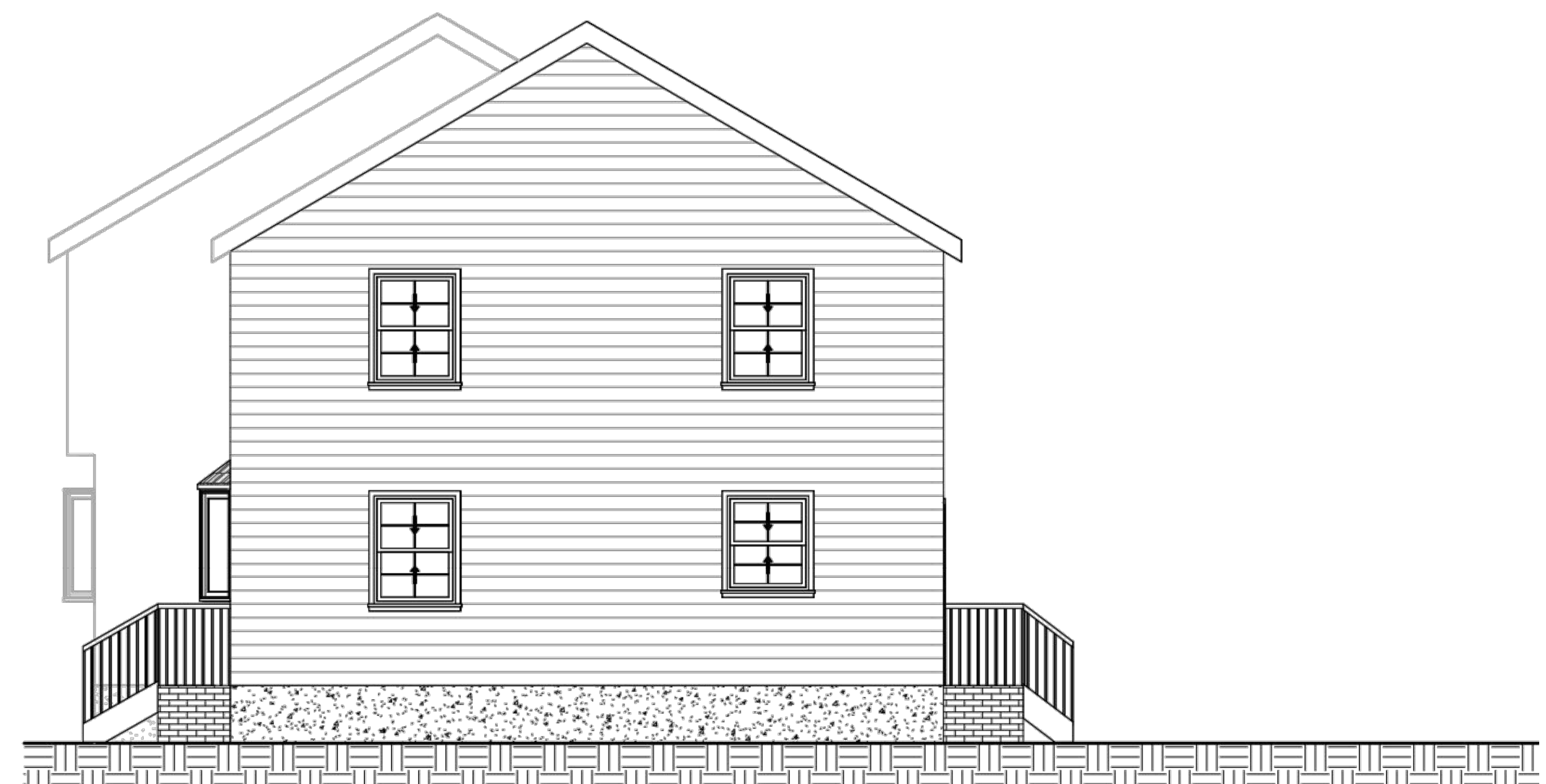
③ RIGHT ELEVATION - EAST ELEVATION 1/4" = 1'-0"
