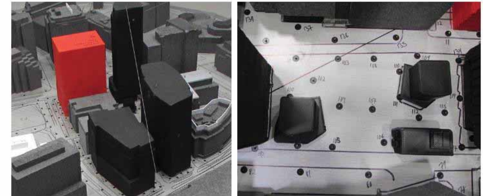
Image 2 - Model of the 105 Broadway Street project as tested in the wind tunnel
