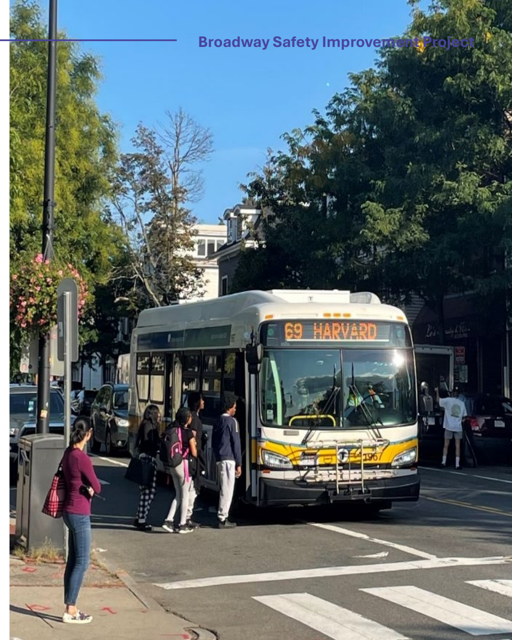
Bus stops that are shorter or before an intersection (as shown) make it harder for the bus to reach the curb. This makes it harder for people to use the accessible boarding ramp, when needed.
