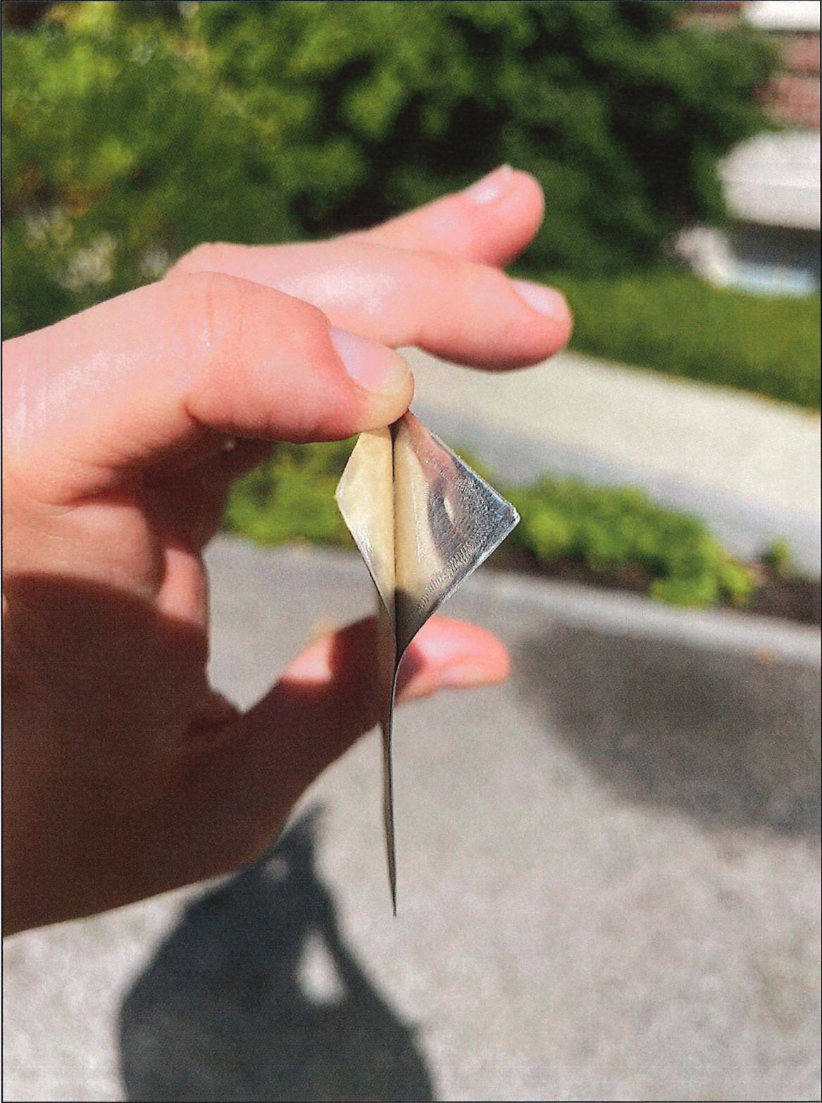
Image 3: Proposed aluminum sign sample for Knafel Center façade. Includes layer of pliable foil and thin layer of pressure sensitive adhesive.
