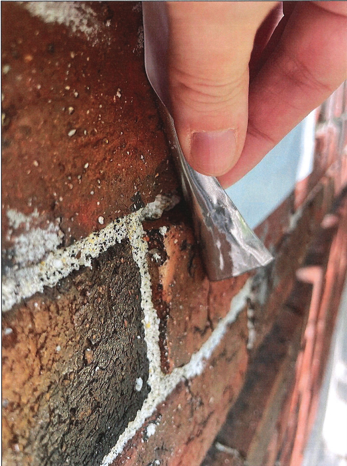
Image 5: Knafel Center south façade test site with sample sign. Removal process includes: 1) Peel off at an angle less than 45 degrees, and 2) Dispose with aluminum recycling.
