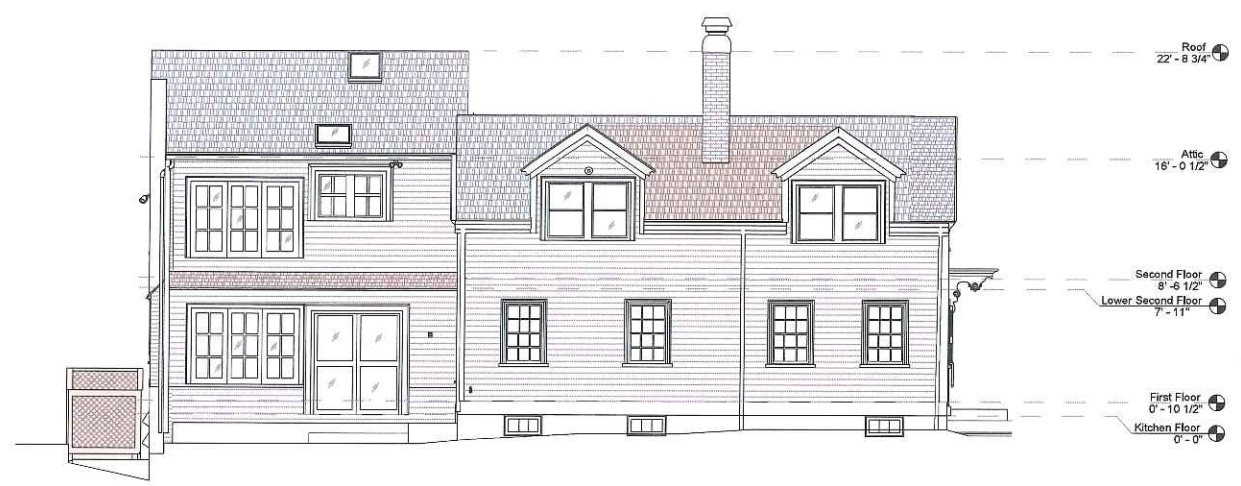
1 Existing East Elevation 3/16" = 1'-0"
