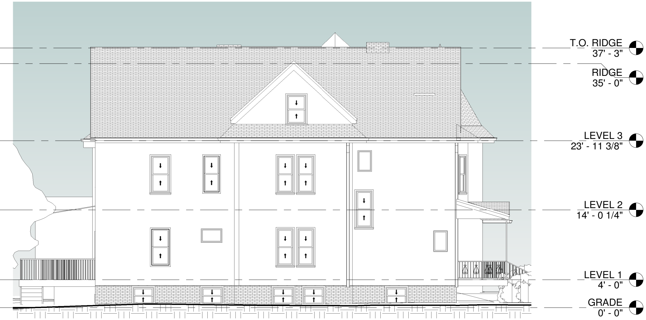
2 BZA EXISTING WEST ELEVATION 1/8" = 1'-0"
