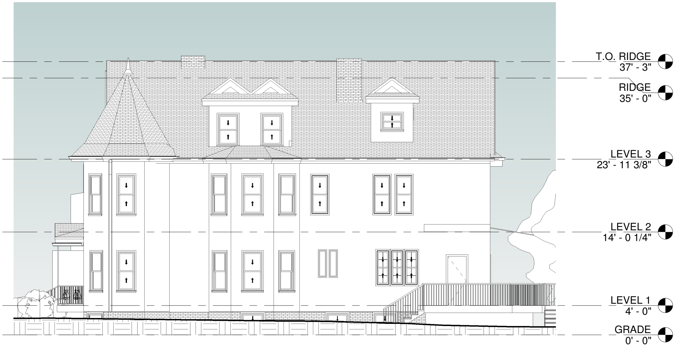
② BZA - EXISTING EAST ELEVATION 1/8" = 1'-0"
