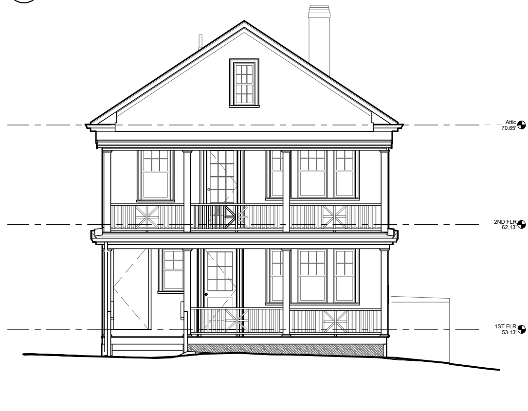
2 FRONT ELEVATIONS (EAST) EXISTING SCALE: 1/8" = 1'-0"
