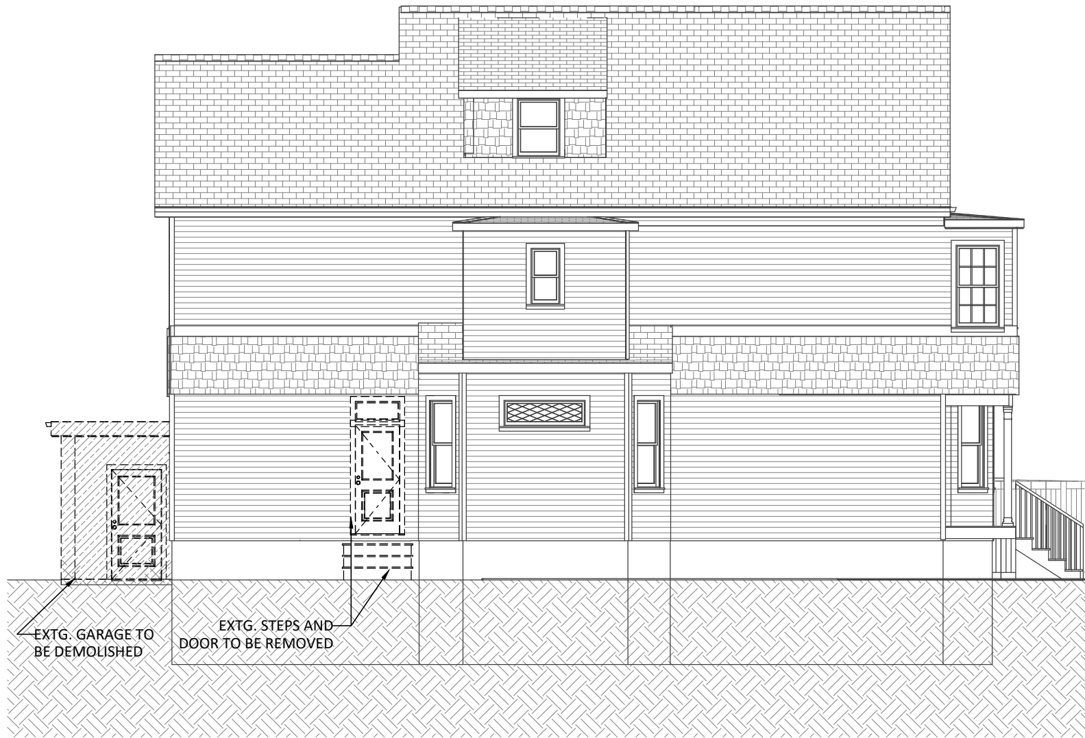
1 LEFT SIDE ELEVATION - EXISTING- 1/8" = 1'-0"
