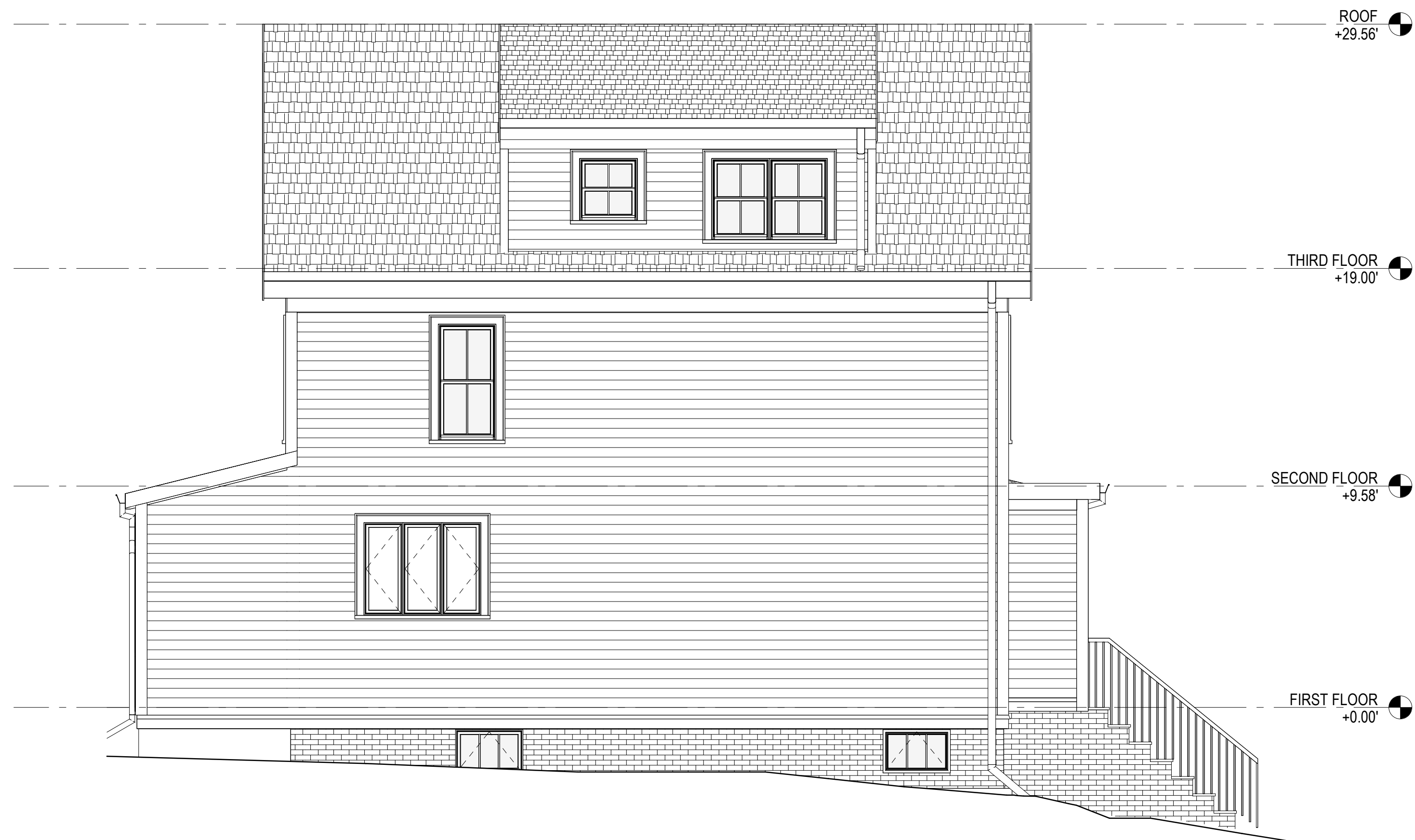
④ WEST ELEVATION - EXISTING SCALE: 1/4" = 1'-0"
