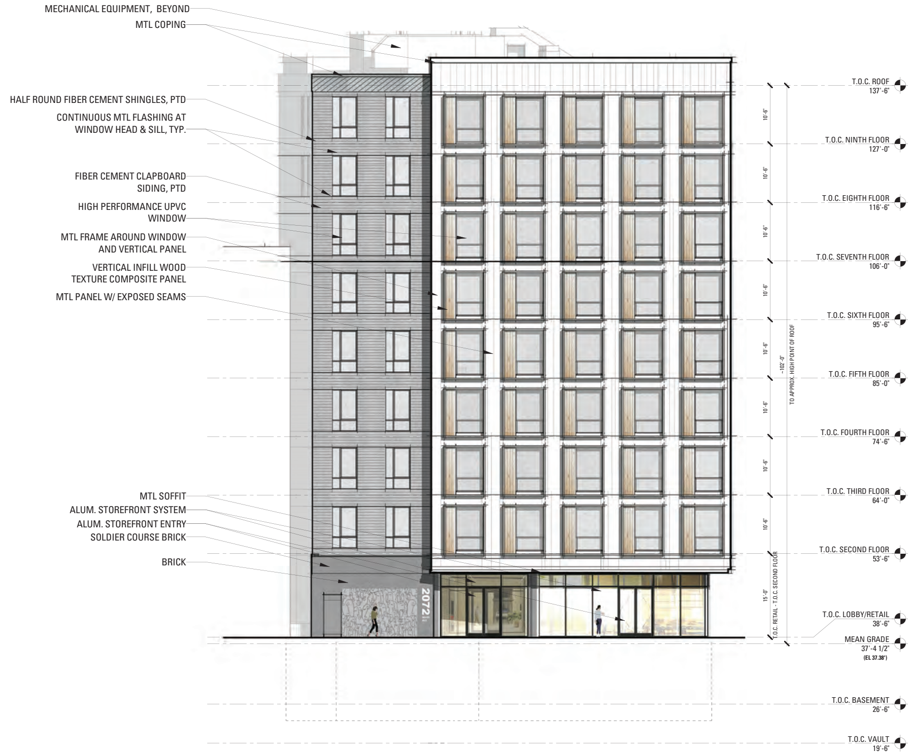
1 BUILDING ELEVATION - NORTH SCALE: 1/8" = 1'-0"
