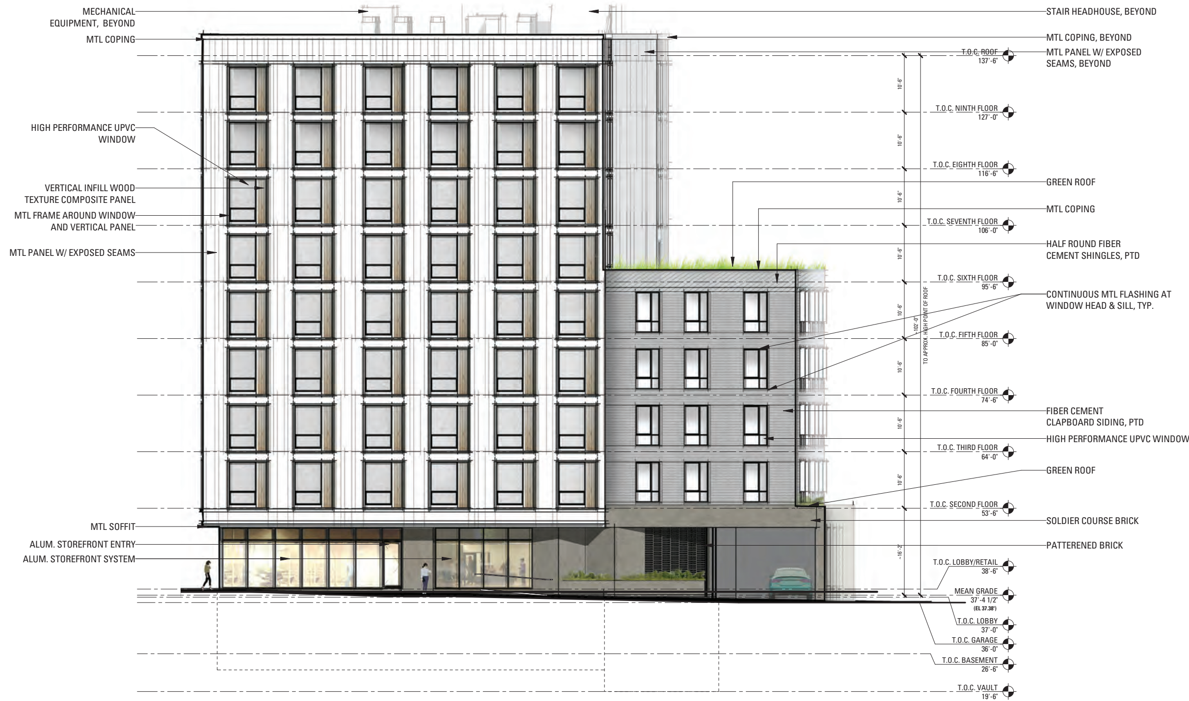
1 BUILDING ELEVATION - WEST SCALE: 1/8" = 1'-0"
