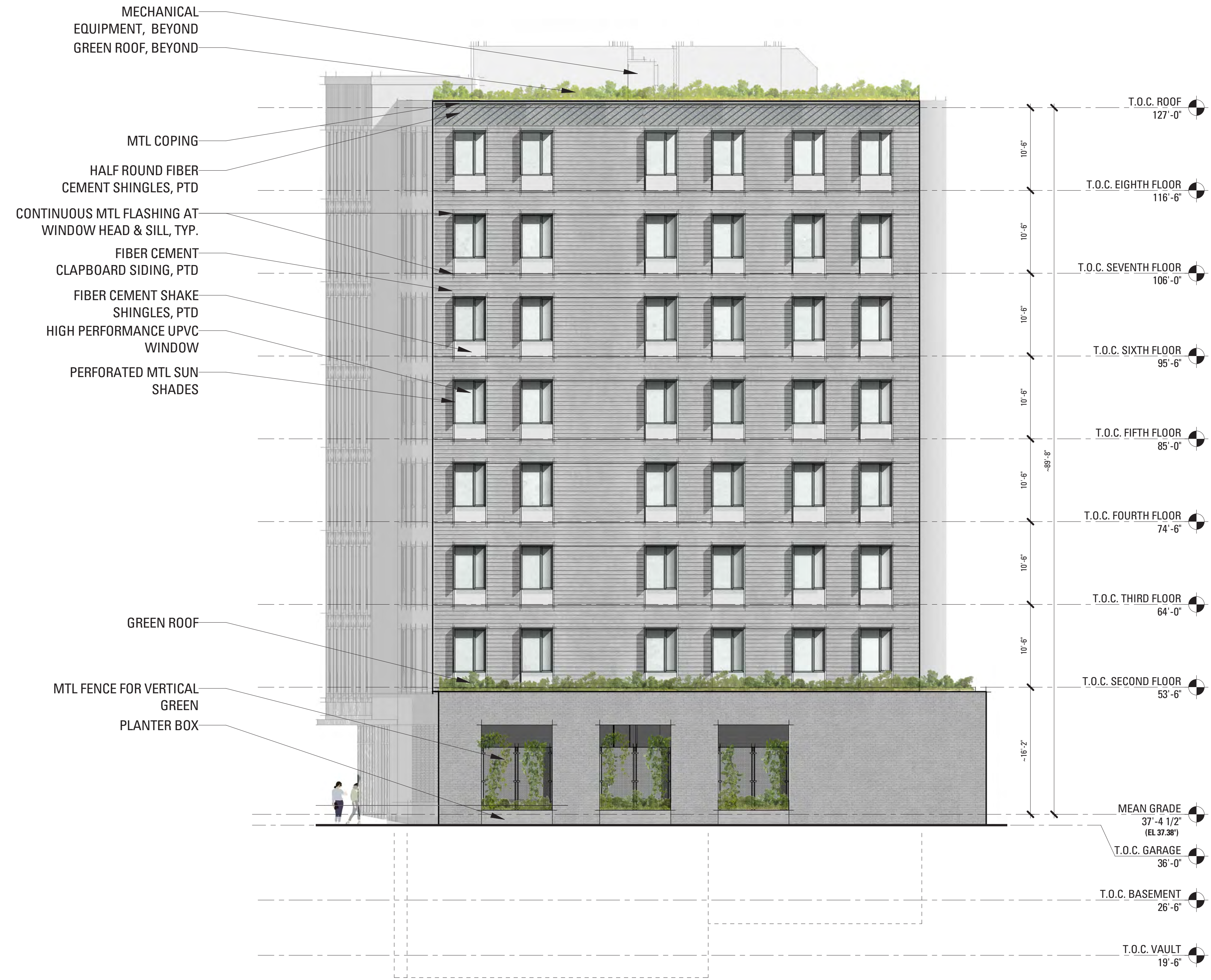
1 BUILDING ELEVATION - SOUTH SCALE: 1/8" = 1'-0"
