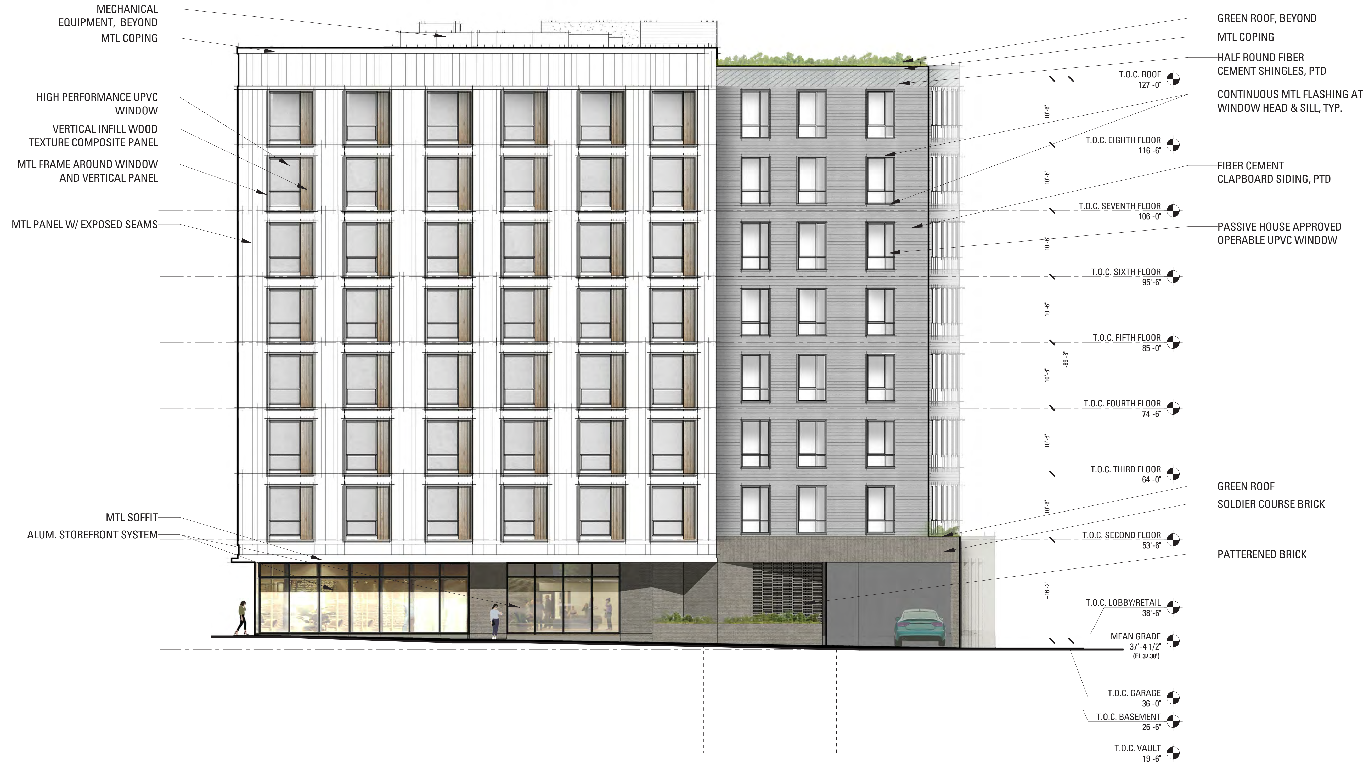
1 BUILDING ELEVATION - WEST SCALE: 1/8" = 1'-0"
