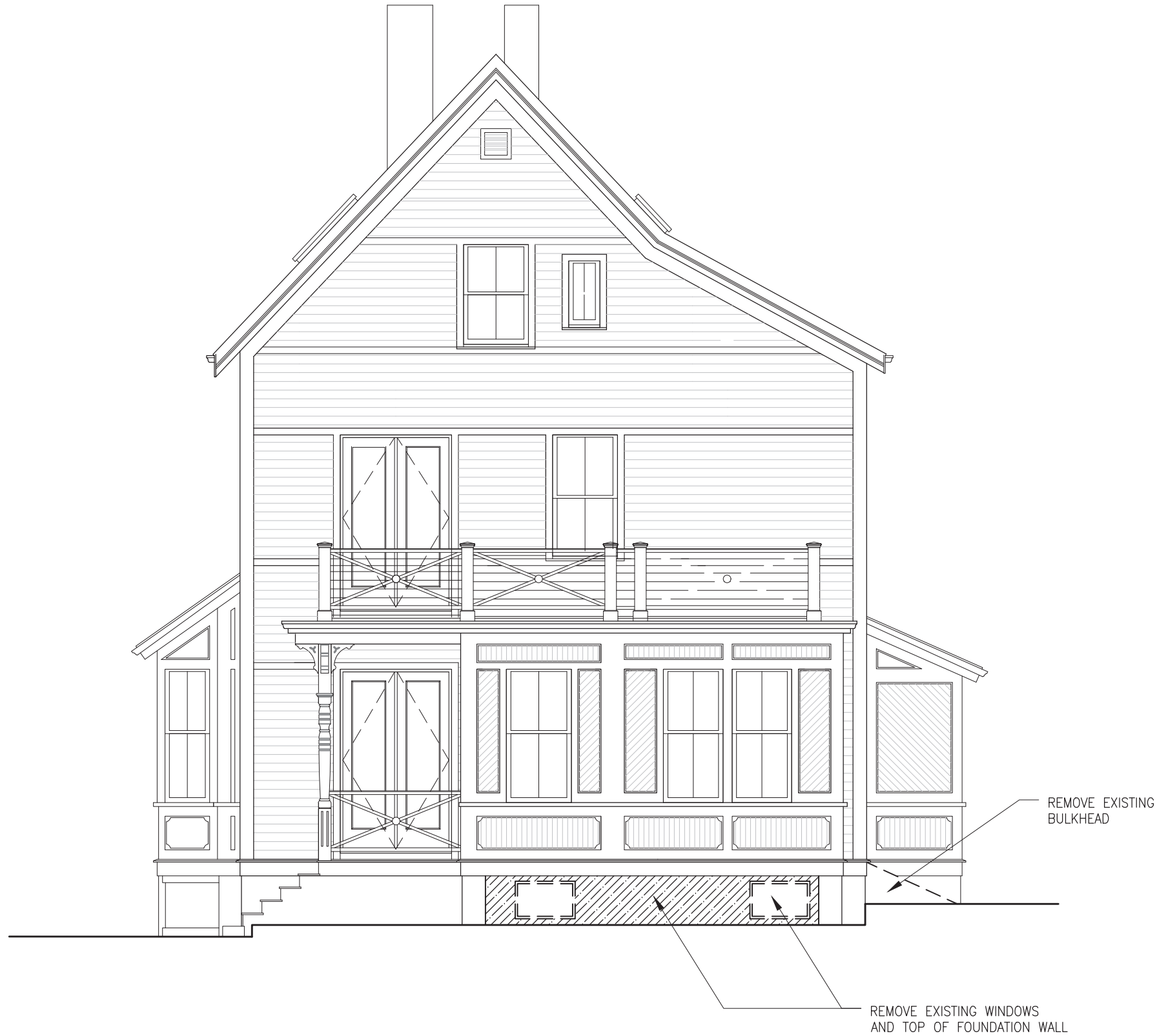
1 REAR (SOUTH) ELEVATION - EXISTING 1/4" = 1'-0"
