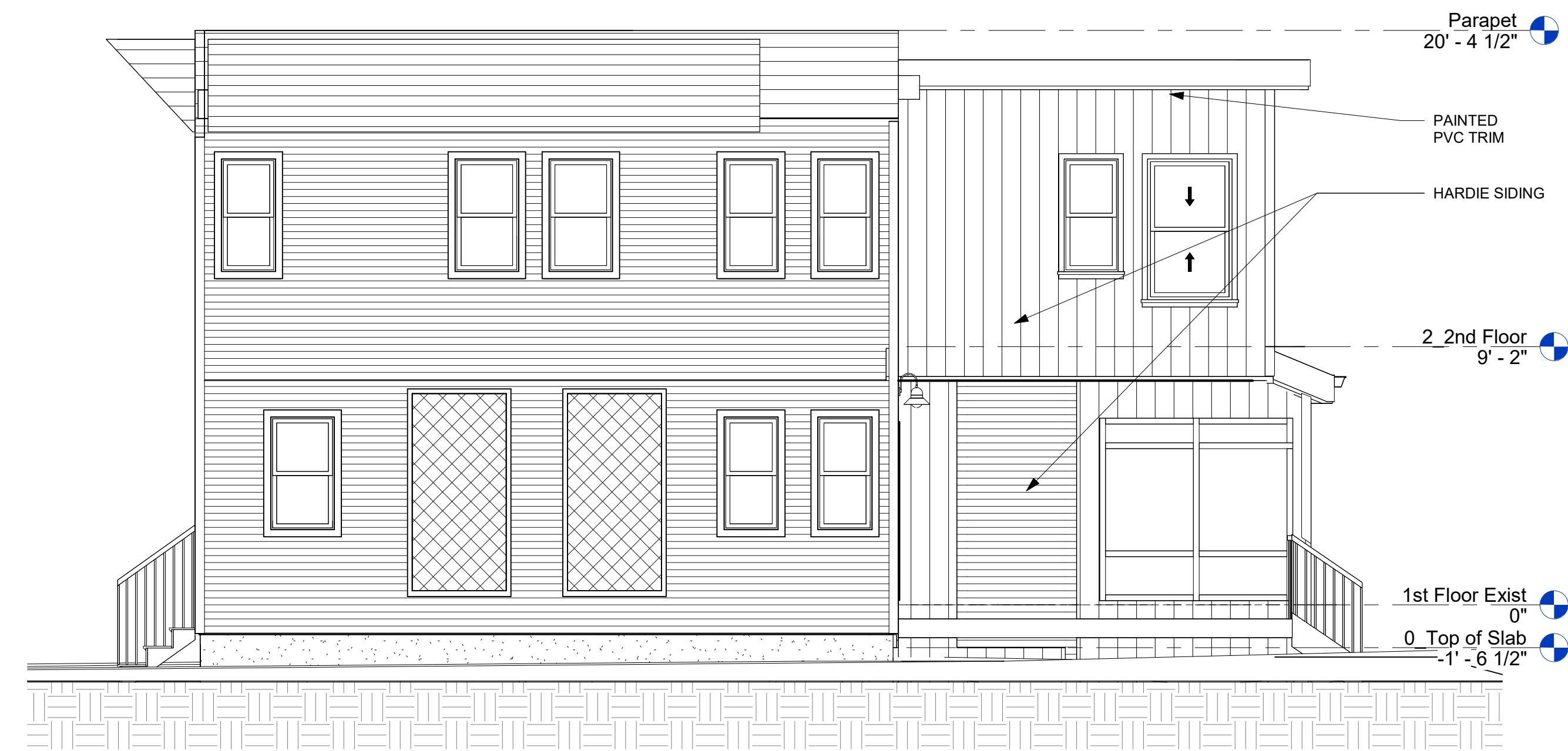
③ Proposed West Elevation 1/4" = 1'-0"
