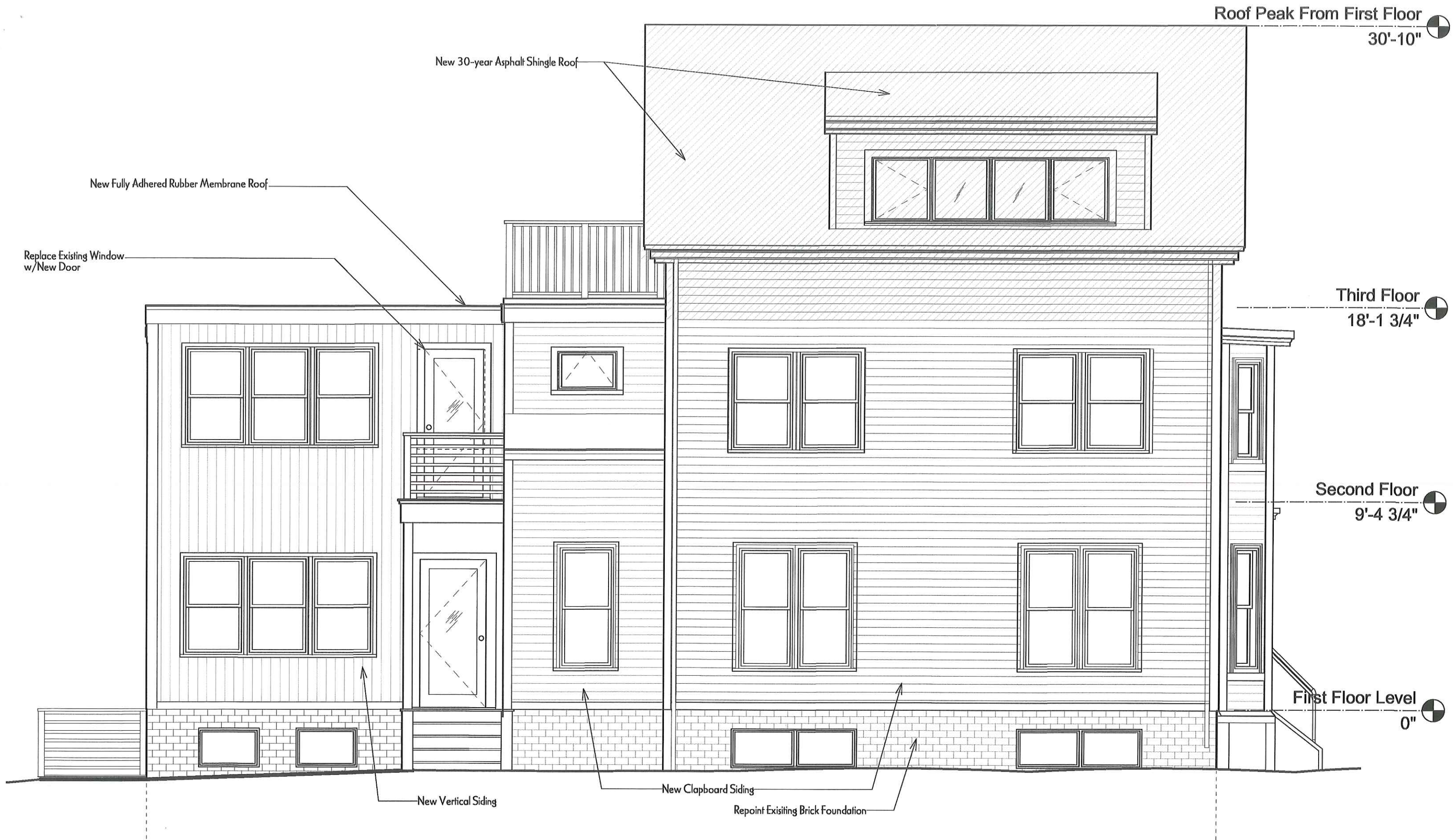
1 Proposed Special Permit South (Side) Elevation OP 2 Scale: 1/4" = 1'-0"
