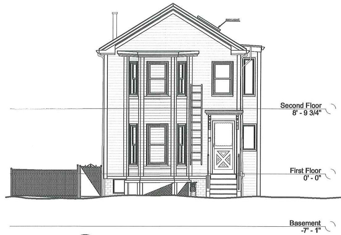
1 Existing East (Front) Elevation Scale: 1/8" = 1'-0"
