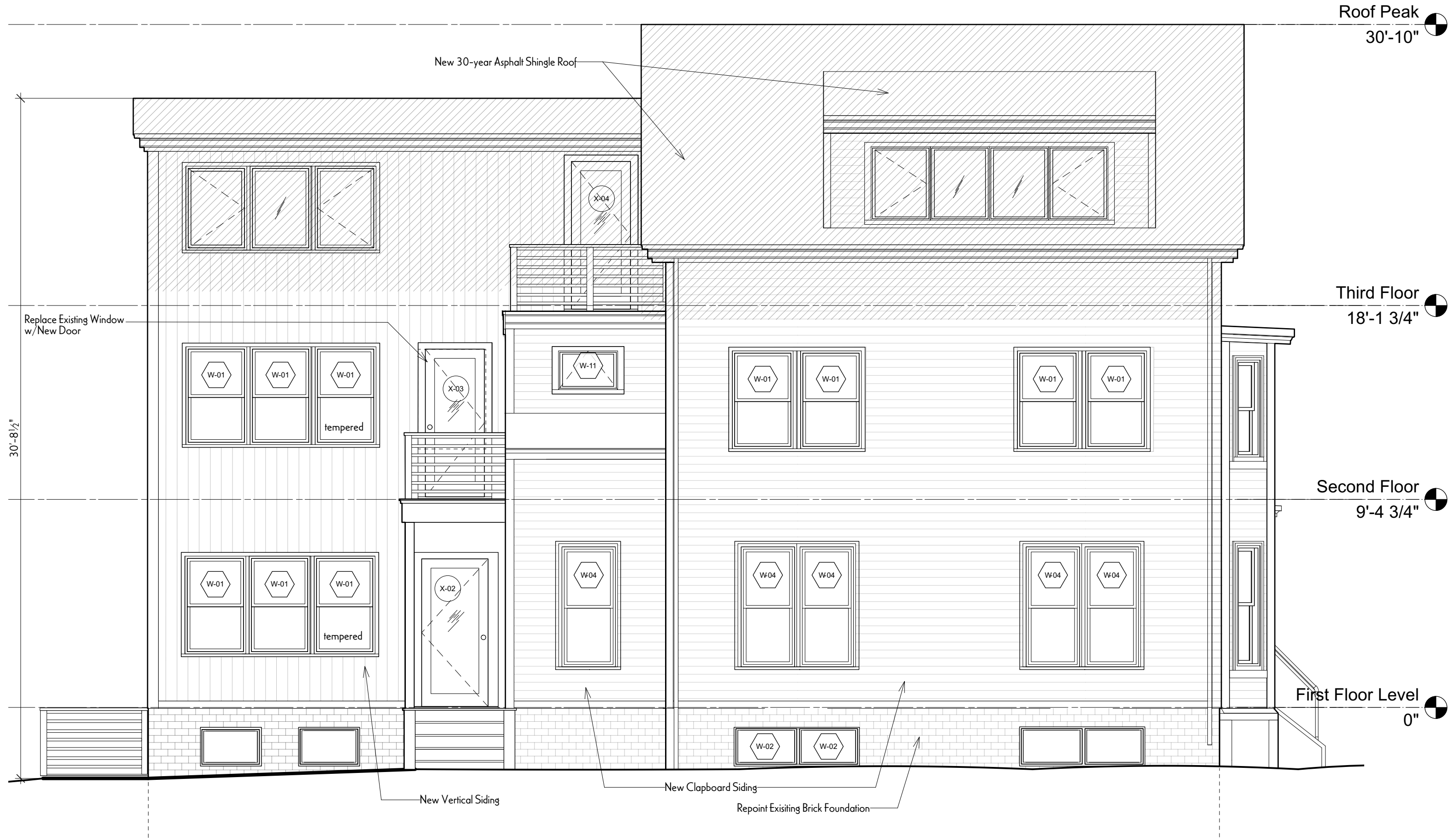
1 Proposed Special Permit South (Side) Elevation Scale: 1/4" = 1'-0"
