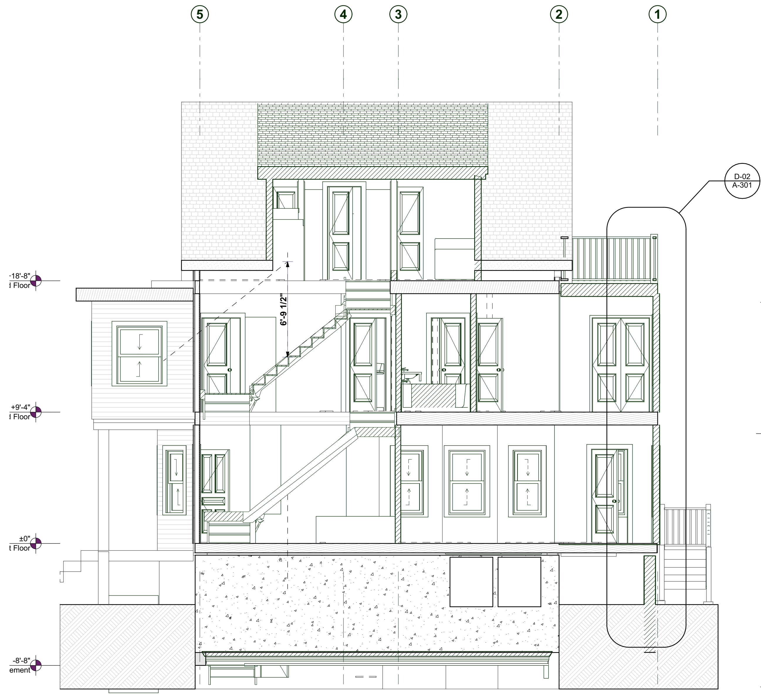
1 Building Section C SCALE: 1/4" = 1'-0"
