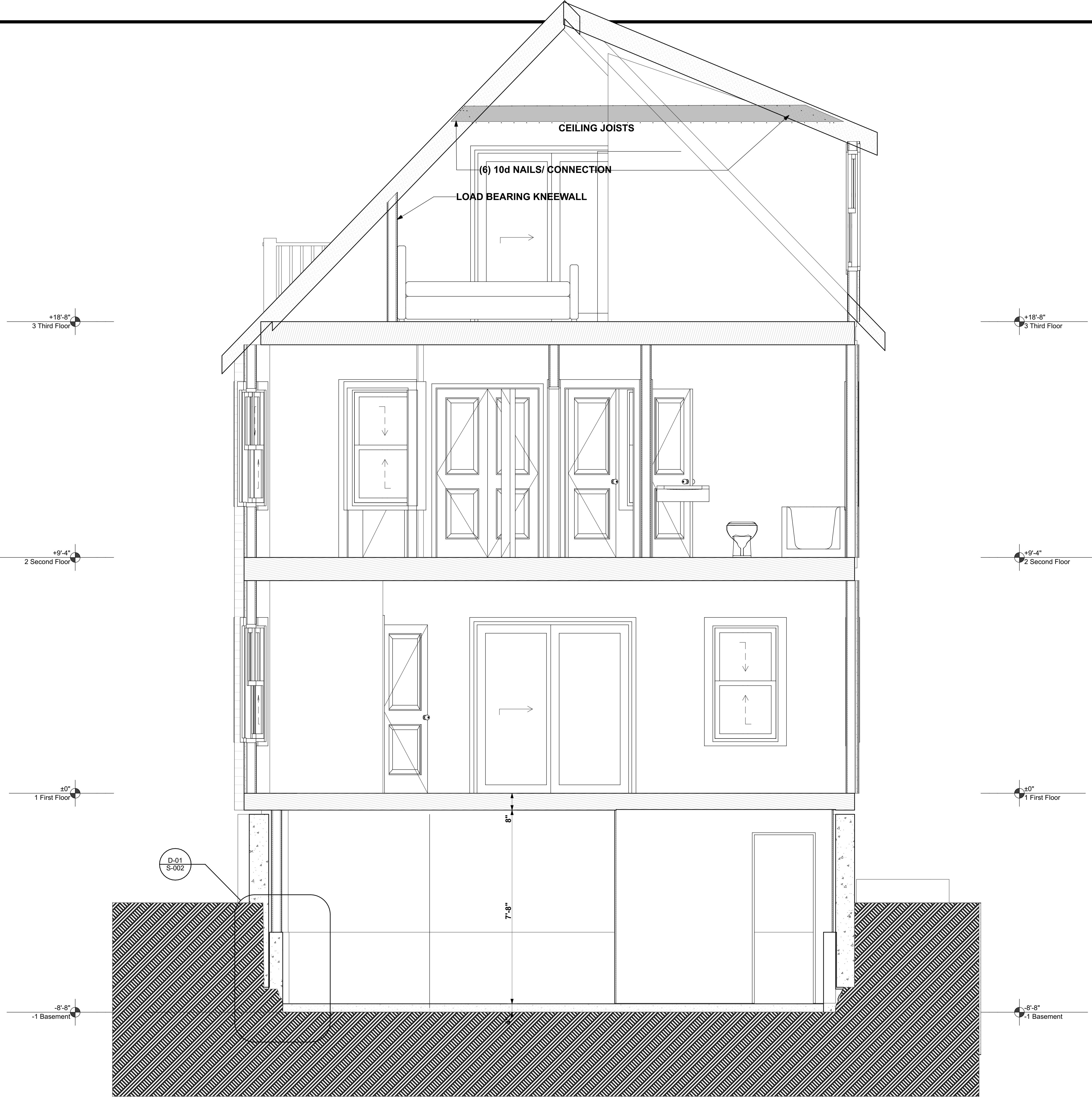
1 SECTION B SCALE: 1/2" = 1'-0" 0 1' 2' 4'
