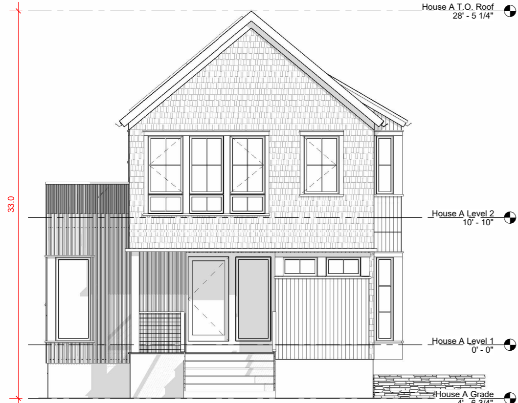
1 House A East Elevation 1/8" = 1'-0"
