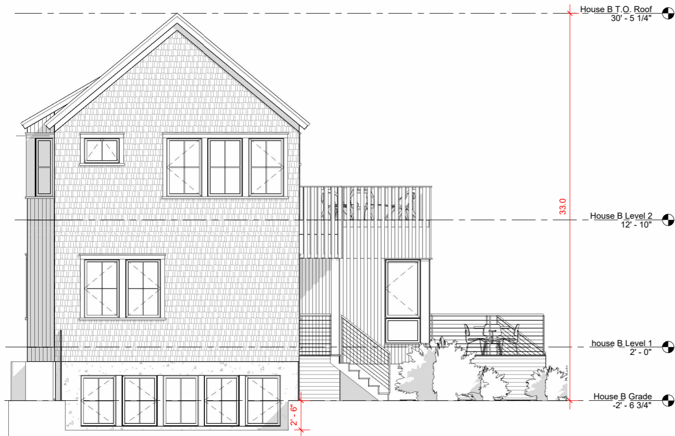
① House B South Elevation 1/8" = 1'-0"
