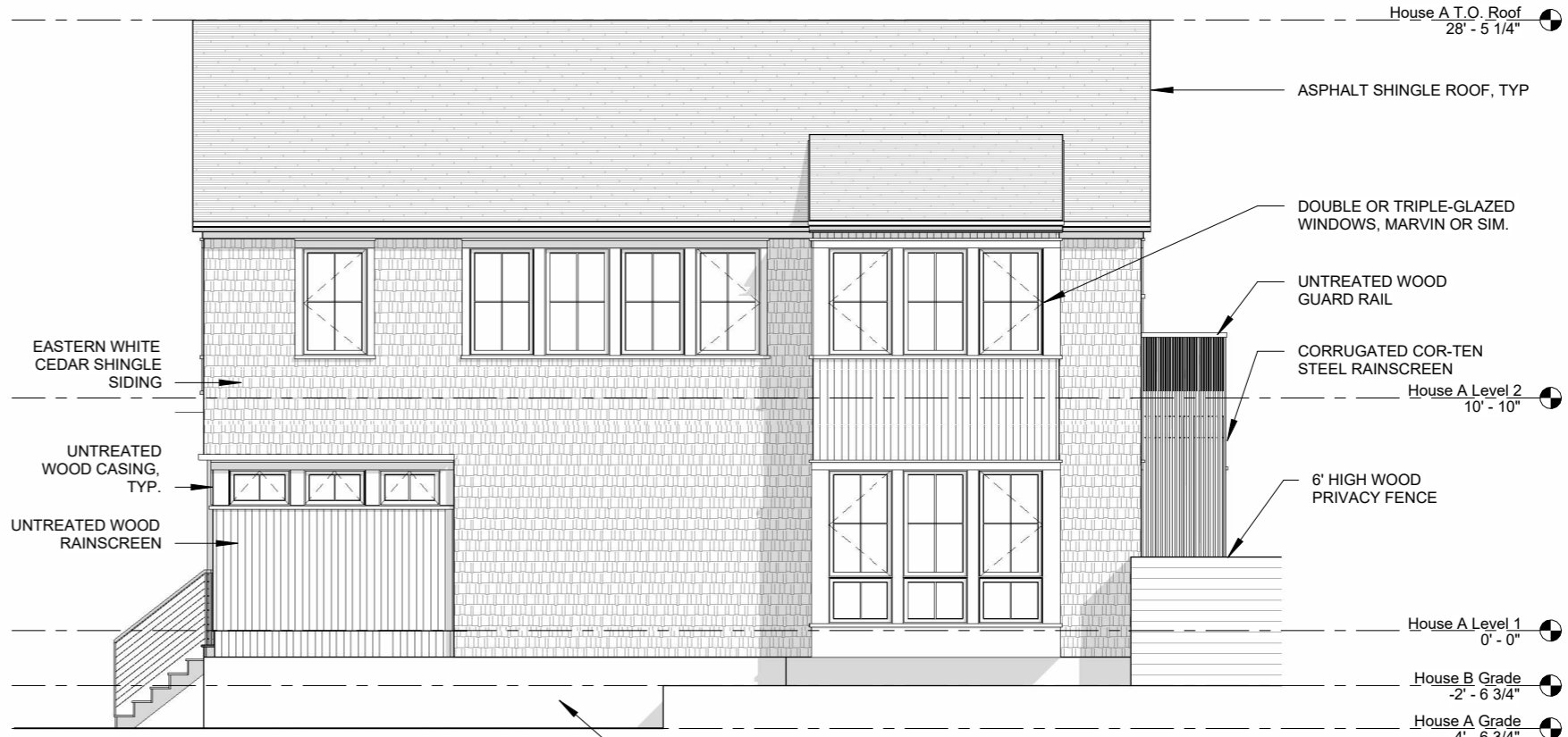
2 House A North Elevation 1/8" = 1'-0"
