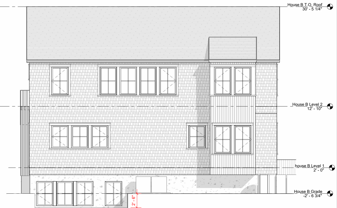
③ House B West Elevation 1/8" = 1'-0"
